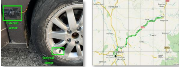
Figure 5: Position of the external and internal sensors on the Scenic (left) and the round-trip journey from Toulouse to Albi, France.
