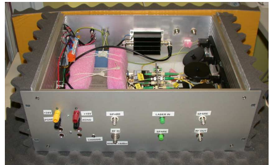
Fig. 4: Laser phase or frequency noise measurement system based on a self-heterodyne interferometer with 2 km delay line [6].
