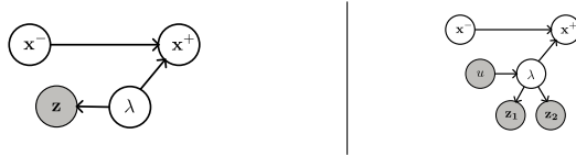
Figure 3.4: Trajectory part between two poses of a pose-graph CBN. \mathbf{x}_{(-)} and \mathbf{x}_{(+)} respectively stand for the past (parent) and the current (child) pose. \mathbf{x}_{(+)} is caused by \mathbf{x}_{(-)} and the relative motion \lambda . (Left) \lambda depends on no external control, and is observed through the random measurement \mathbf{z} . Note that a prior on \lambda may exist. (Right) The external control input u causes \lambda through a conditional probability distribution (CPD), and \lambda gives rise to multiple measurements (limited to 2, \mathbf{z}_1, \mathbf{z}_2 , but the approach can be generalized).
