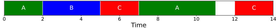
Fig. 1. In this toy example, we have 3 jobs (A,B,C), with \underline{m}_A = 1 , \overline{m}_A = 3 ; \underline{m}_B = \overline{m}_B = 1 ; \underline{m}_C = \overline{m}_C = 2 . Job A is the only one with variable duration, \underline{p}_A = 2 , \overline{p}_A = 4 . The only precedence constraint is (A, B) , so at least k tasks of job A must occur before the k -th task of job B. We have lag_A^{min} = 5 and lag_C^{max} = 5 . T_B = \{2\} , so the only task of job B must start at t = 2 . In this example, the objective is to maximize the number of tasks for job A first ( u_A = M , with M a large number), then we want to maximize the total duration for A ( v_A = 1 ). For the other jobs i \neq A , we have u_i = v_i = 0 .
