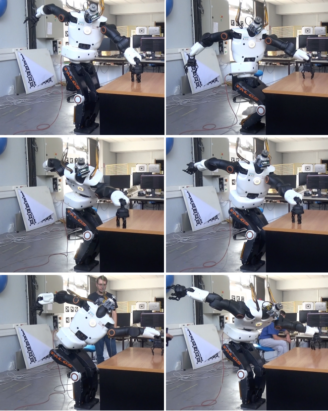
Fig. 5: Experimental setup showing TALOS making 3-points contacts between its gripper and a flat table while maintaining balance and fixed feet on the ground.
