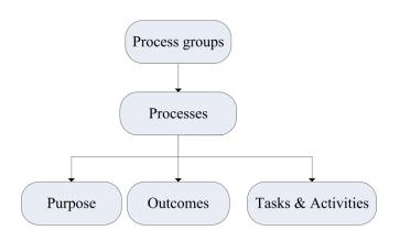
Figure V-1 Structure of ISO/IEC 15288
