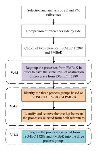
Figure V-11 The proposed method of harmonization of PM and SE processes
