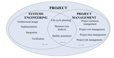
Figure II-2 Overlaps between SE and PM based on (Kossiakoff et al. 2011)
