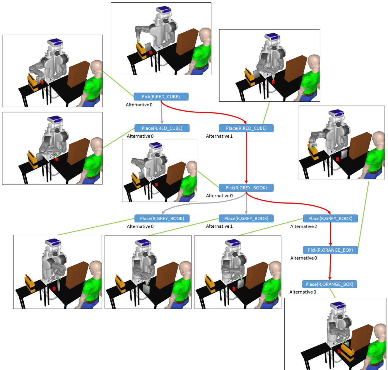
FIGURE 3.16: The different steps of a geometric plan, including the unused alternatives. In the plan, the robot performs three successive Pick and Place on three objects.
