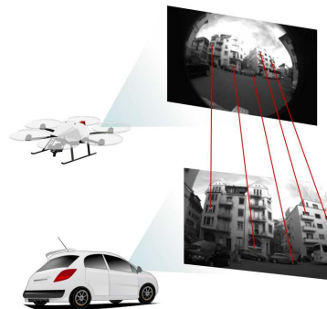
Figure 1: In an effort to move towards robust mapping and localization in unconstrained environments, this paper investigates graph comparison approaches to visual place recognition. Structural and visual information provided by covisibility graphs is combined, in order to cope with variations and noise in observations, such as those coming from heterogeneous teams of robots.
