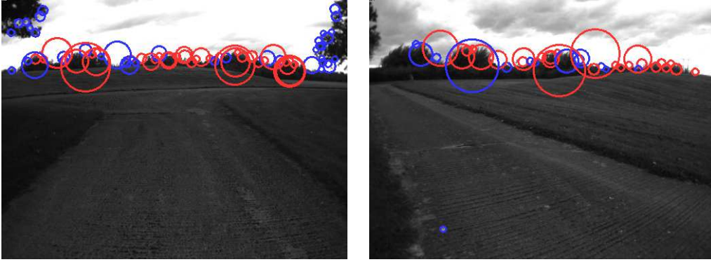
Figure 4.4: Examples of images from the Begbroke sequence which correspond to the regions of confusion in first matrix of Figure 4.3, due to their non-discriminative appearance. The images contain many matched visual words (shown in red), despite depicting different locations. However, these locations tend to produce low matching probabilities regardless, which indicates a low confidence due to common appearance.
