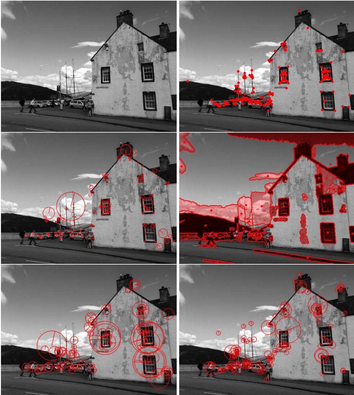
Figure 2.6: Examples of various interest point detectors: original image (top-left), Harris corners (top-right), SIFT (middle-left), MSER (middle-right), SURF (bottom-left), and BRISK (bottom-right).
