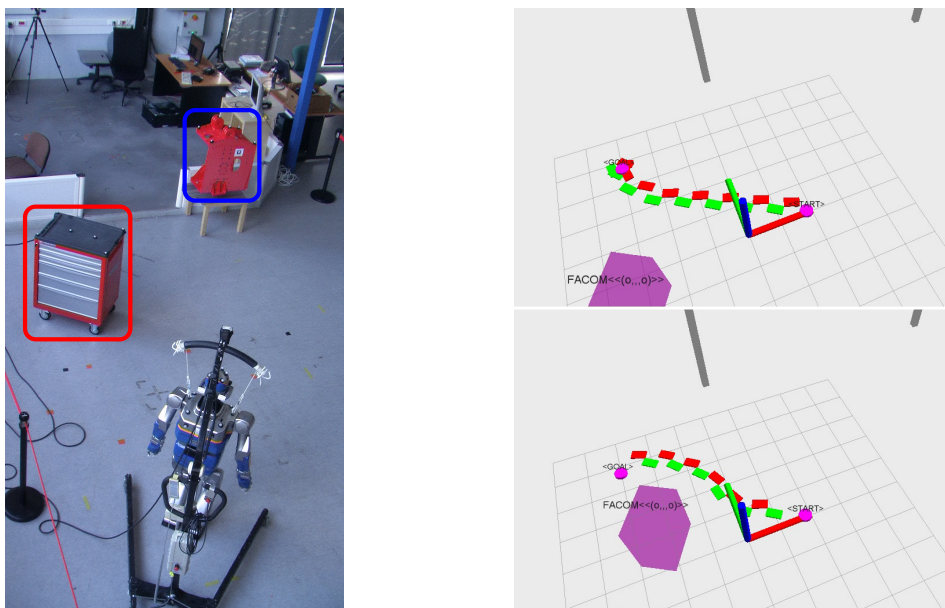
Figure 6.1: Situation of the experiment: The robot has to go in the vicinity of the pylon engine depicted in blue in the left picture while avoiding the red moving toolbox. The top right picture show the first planning and the bottom right the re-planned trajectory after the tool box got into the way.
