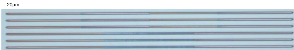
Figure 2.19: Example of 2 μm width step channels written with 1 beam passage.
