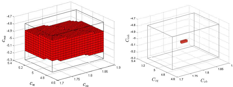
Figure 4.2: Admissible  $C_{z\dot{\alpha}}$ ,  $C_{zq}$ ,  $C_{m\dot{\alpha}}$  with constant (left) and optimal (right) inputs
