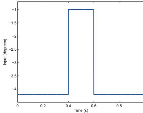
Figure 4.1: Optimal input obtained via the set-membership-T-optimality criterion
