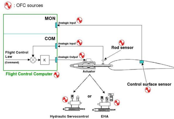
Figure 6.1: OFC source location in the control loop.
