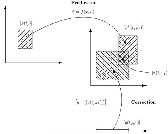
Figure 6.6: Prediction-correction step at time  $t_j$ .
