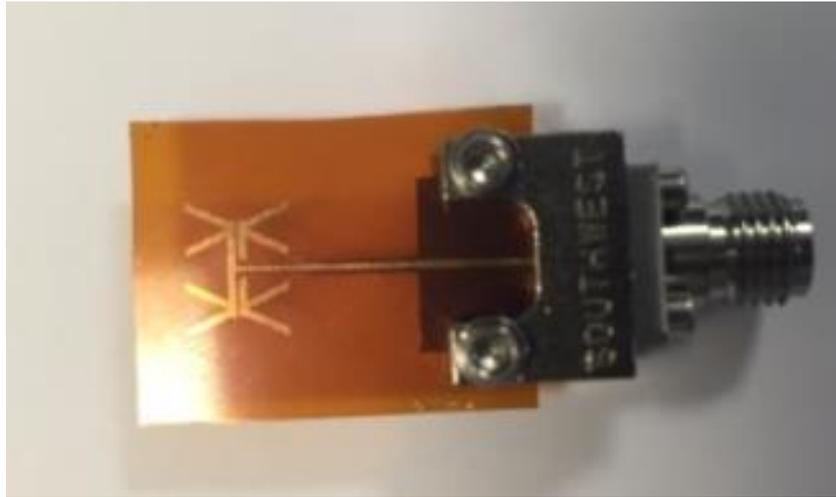
Figure III.17: Manufactured Cross dipoles array antenna.
