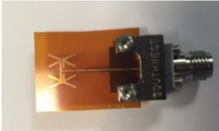
Figure III.17: Manufactured Cross dipoles array antenna.
