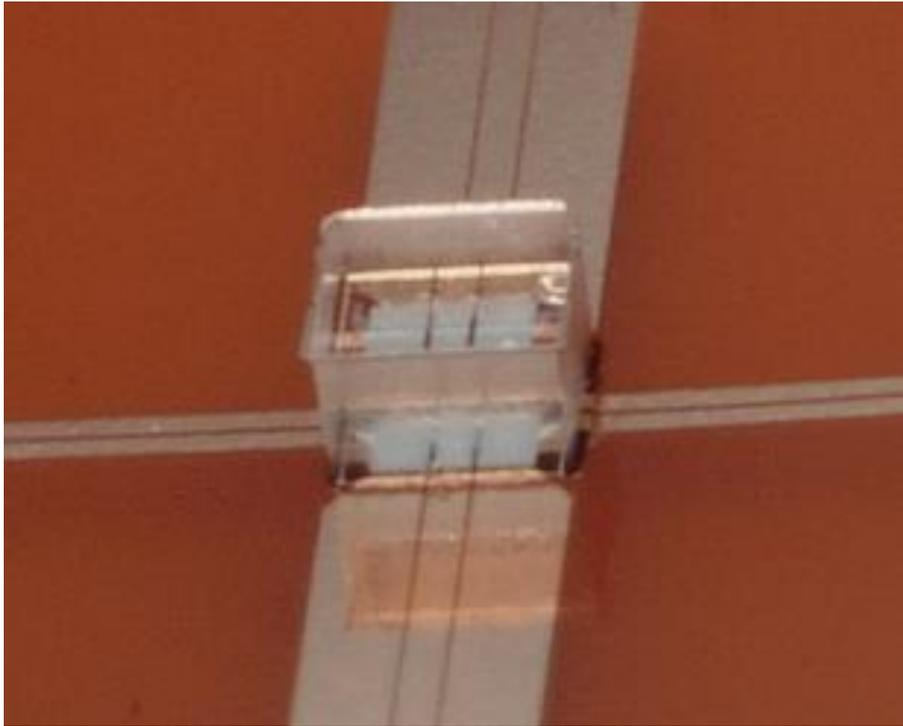
Figure V.13: Photograph of LNA dummy mounted on Kapton.
