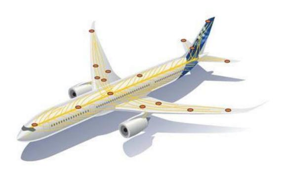
Figure I.1: Structural health monitoring (SHM) systems arrayed in keay areas where loads are highest. Source: Airbus
