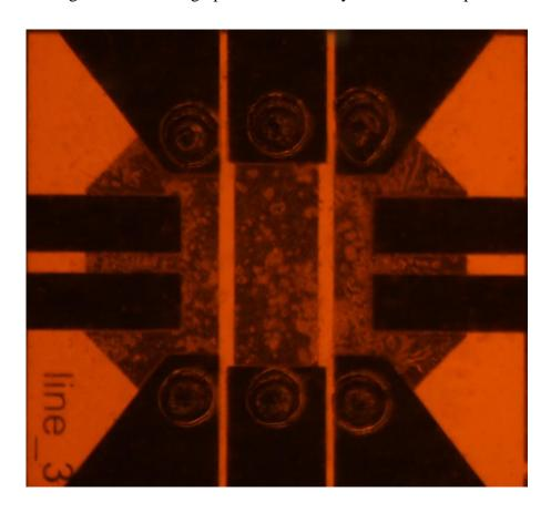
Figure V.14: Bottom view (through Kapton) of a LNA dummy mounted by the flip chip technique.
