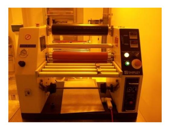
Figure III.3: Shipley 360N Laminator.
