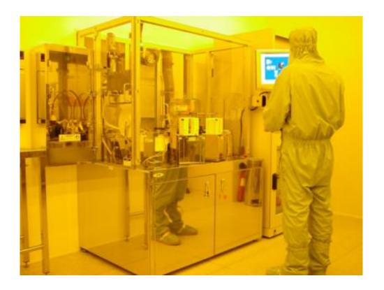
Figure III.4: EVG120 resist processing system.
