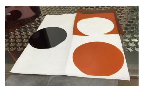
Figure IV.3: Cut Kapton tape into a 4-inches wafer shape.
