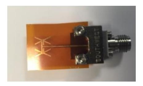
Figure III.17: Manufactured Cross dipoles array antenna.
