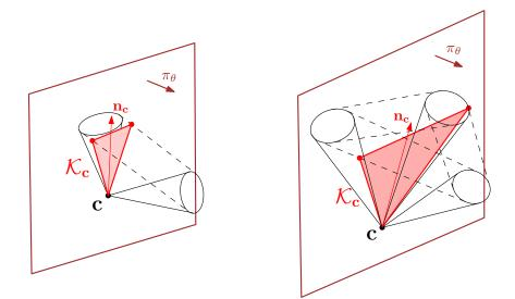
Figure 6.1: Two examples of intersections between a convex-cone and a vertical plane, for two (left) and three (right) summed cones.
