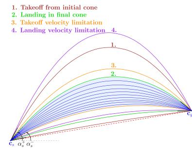
Figure 5.8: Illustration of the constraints on a practical example: each constraint bound is used as  $\alpha_s$  and represents a bold parabola. Between these bounds, the constraint is satisfied, out of them not. The constraint intersection is given by the bounds  $(\alpha_s^-, \alpha_s^+)$  and illustrated by the gray zone: blue parabolas belonging to it are admissible solutions to the problem.
