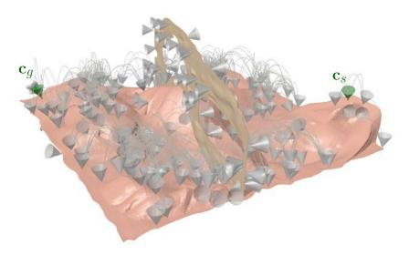
Figure 5.10: Preliminary result of a roadmap generation in a desert environment. Nodes are represented by their friction cones.
