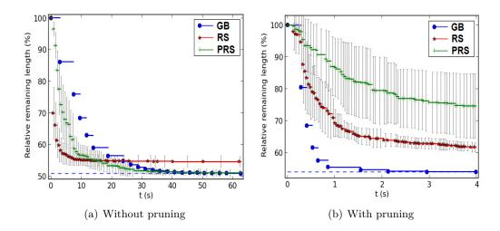
Figure 3.11: Influence of a pruning step on the optimization processes. RRT-connect provides an initial path with 62 waypoints, which is downed to 2 waypoints by Prune. Concerning the path length, it is only reduced of 6.2% by Prune. Thus, final path lengths provided by GB in both cases are equivalent, the major difference results in the computation time of GB.
