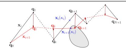
Figure 3.3: Illustration of one iteration of the path optimization.  $\mathbf{x}_{i+1}$  appears to be in collision with the obstacle. The first colliding configuration  $\mathbf{x}_{i+1}(\kappa_i)$  at abscissa  $\kappa_i$  is returned by the continuous collision checker. The corresponding constraint will be computed in the backtracked configuration  $\mathbf{x}_i(\kappa_i)$ .
