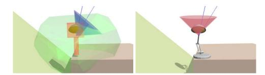
Figure 6.7: Different contact cones for the jumping lamp. (Left) The blue cone comes from the intersection between the  $\mathbf{W}^k$  shape and the left surface, and is moved to the COM of the reduced lamp model. It is used to validate the non-sliding constraint during the planning stage. (Right) The red cone is the friction cone from the contact on the right surface, moved to the COM. As the parabola lies inside the red cone, this configuration satisfies the non-sliding constraint.
