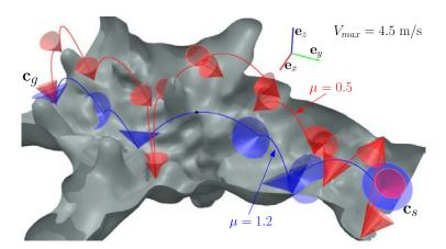
Figure 5.14: Path planning results in a cave. The robot has to avoid the numerous stalactizes, stalagmites and holes. Number of triangles: 33513.
