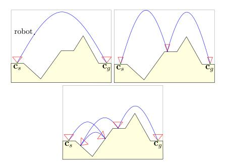
Figure 5.1: Three sequences of parabolas between  $\mathbf{c}_s$  and  $\mathbf{c}_g$  positions for different constraints. In the case illustrated on the right, friction cones are narrower than those on the left, so that the parabola on top is not admissible anymore, and a waypoint has to be used. In the bottommost case, the initial velocity has been limited compared to the left case, resulting in a sequence with numerous jumps.
