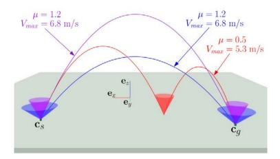
Figure 5.9: Three parabola examples linking  $\mathbf{c}_s$  to  $\mathbf{c}_g$  with different constraints. Large (blue) and narrow (violet) friction cones are considered, forcing the solution parabola to be adapted. With a large velocity limitation,  $\mathbf{c}_g$  can be directly reached (blue). Otherwise, an intermediate position has to be considered (red).
