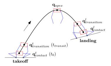
Figure 6.10: Key configurations computed along a parabola trajectory.
