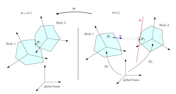
Figure 3.4: Bodies representation in collision-configuration (left) and backtracked collision-free configuration (right). A contact point (i.e. any point in the intersection of the bodies)  $\mathbf{P}_c$  can be returned by the Flexible Collision Library [Pan 2012a], used to detect collisions. Constraint defined by Equation (3.4) aims at keeping  $\mathbf{P}_2(\mathbf{q})$  in plane II fixed to  $\mathcal{B}_1$ .
