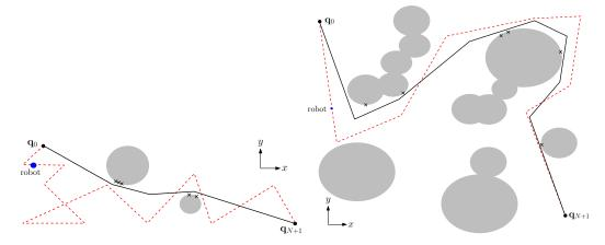
Figure 3.7: Path-optimization results on 2D robots, moving around gray obstacles. Initial paths are dashed and crosses represent contact points  $\mathbf{P}_c$  related to collision-constraints. Note that, on the left, the detour completely disappears.
