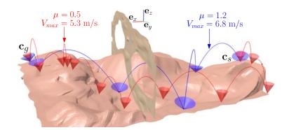
Figure 5.12: Full path planning results in an environment containing two windows to cross from right to left. The red solution is more constrained, so it results in a longer sequence of parabolas. Number of triangles: 47733.
