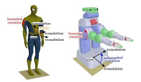
Figure 2.3: Examples of joints for a humanoid character and the PR2 robot.
