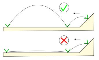
Figure 5.5: Illustration of the conservative non-slipping condition. (Top) The trajectory is valid, since landing and takeoff velocties are included in the centroidal green cone. (Bottom) The trajectory is found invalid by our criterion.
