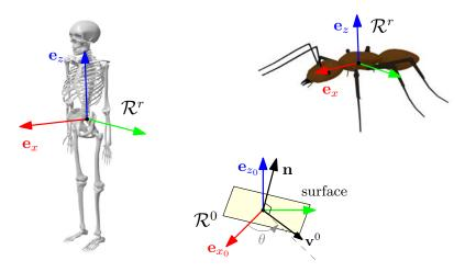
Figure B.1: Local frame definitions for a humanoid (left) and a non-humanoid character (right).  $\mathbf{v}^0$  is the desired facing direction, given a surface normal  $\mathbf{n}$  and an orientation angle  $\theta$ .
