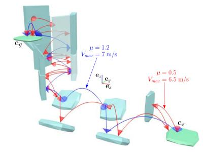
Figure 5.13: Full path planning results in an environment containing platforms and a chimney. The blue path is constrained by large cones, the red path by narrow cones. Reducing  $\mu$  prevents the creation of a parabola linking two low platforms with the same inclination. Number of triangles: 696.
