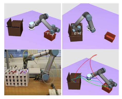
Figure 3.8: (Bottom left) An industrial use-case example proposed by Philips for the Factory-in-a-Day project<sup>3</sup>. A similar environment has been created (top) to illustrate that our method can comply with an industrial problem, where initial and final configurations of the UR5 are constrained in boxes. End-effector trajectories are illustrated (bottom right): RRT planning in red, a RS optimization in blue, a PRS one in cyan and the GB optimization in green.
