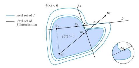
Figure 3.5: Illustration of linearly constrained quadratic program on an analogous problem to the path shortening problem. Iterations  $\mathbf{x}_i$  are represented for  $\alpha_{init} = 0.25$ . The nonlinear constraint is defined as  $f(\mathbf{x}) \leq 0$  and the linearized ones as the  $L_i$  lines. The bottom right picture shows a condition for the linearized constraint  $L_1$  to be linearly dependent on  $L_2$  by being stationary at the boundary of f.
