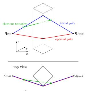
Figure 3.2: Example of a path in  $\mathbb{R}^3$ . The optimal path belongs to the x - y plane containing  $\mathbf{q}_{init}$  and  $\mathbf{q}_{final}$ . Random shortcut will never manage to optimize the initial path: each shortcut attempt will provide a collision.
