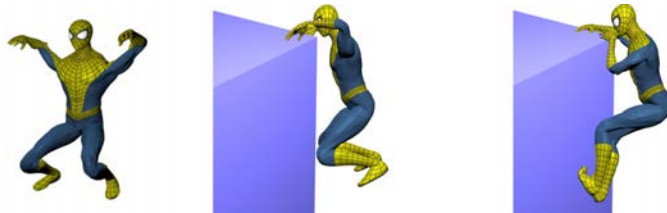
Figure 6.6: Illustration of the generation of a contact configuration. (Left) The manually defined reference configuration. (Middle) The root of the reference configuration is placed close to an obstacle so that the obstacle is in the accessible space of the limbs. (Right) Result of the configuration projection on the obstacle to create contacts with the hands and the feet.
