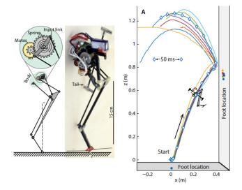
Figure 4.2: Robot presented by [Haldane 2016], and trajectories obtained when jumping from the ground to a vertical wall.
