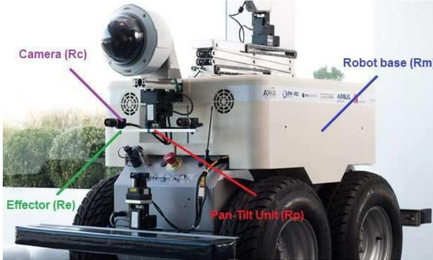
Figure 3.1.: Air-Cobot and the associated frames [Demissy et al., 2016]
