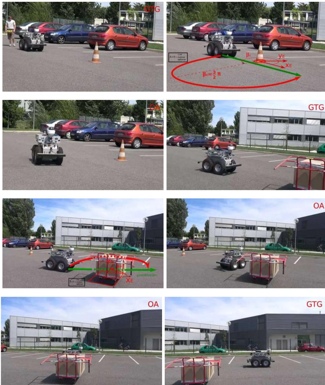
Figure 4.20.: Extract of video sequence - static obstacles
