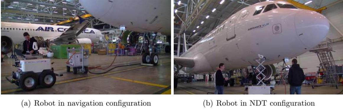
Figure 2.18.: Picture of Air-Cobot in default configuration and with the pantograph-3d-scanner unit extended for inspection
