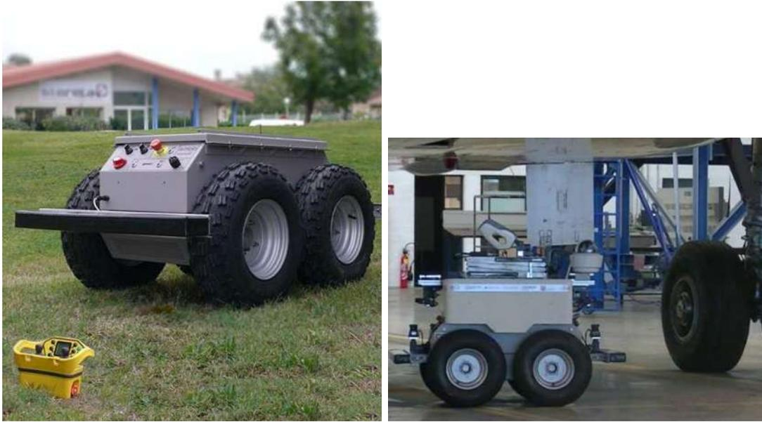
(a) Robot platform, 4MOB, designed by Sterela (b) Robot platform fully equipped during an experimental test run next to an A320
