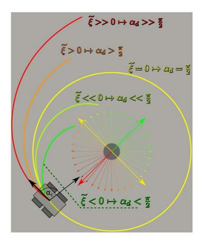
Figure 4.8.: Visualization of spiral obstacle avoidance extension for moving obstacles
