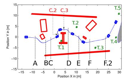
Figure 4.18.: Avoidance Experiment for static Obstacles
