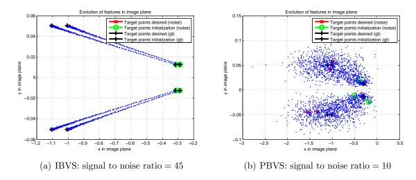
Figure 3.17.: Evolution of features in a noisy simulation
