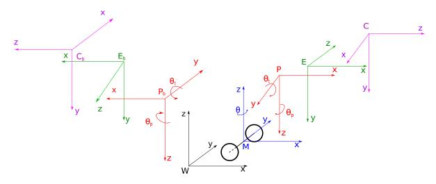
Figure A.2.: Robot coordinate system for the rear cameras
