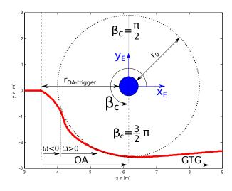
Figure 4.24.: Successive robot positions - Close up of first OA
