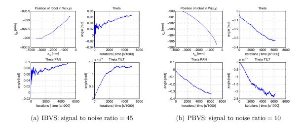
Figure 3.18.: Robot path, orientation and camera state in a noisy simulation
