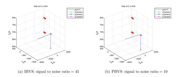
Figure 3.16.: Evolution the point C (camera origin) in a noisy simulation
