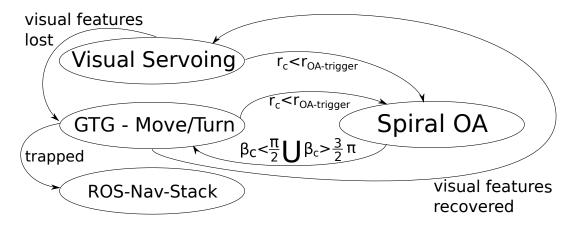
Figure 2.20.: Schematic of the state machine which defines the decision process
