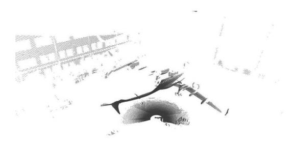
(a) 3d scan acquired with Hokuyo during experimentation on Airbus 320 - robot pose behind the wing
