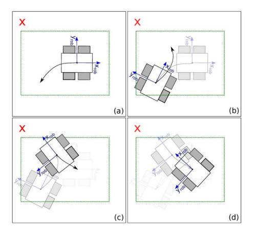
Figure 2.16.: Modification of the align first behavior to decrease tire wear.
