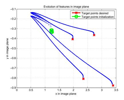
Figure 3.12.: Evolution of features in a PBVS simulation
