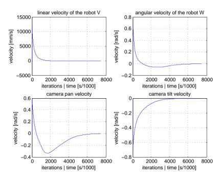
Figure 3.9.: Evolution of velocities in a IBVS simulation
