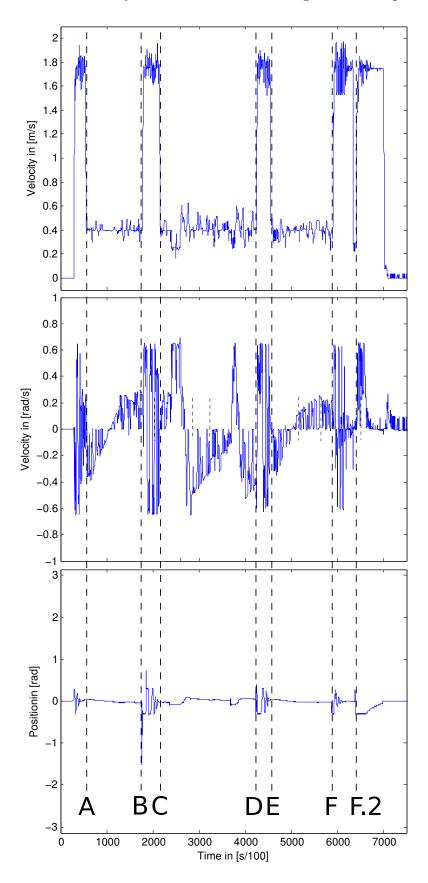
Figure 4.19.: Robot linear and angular Velocities and Camera Angle
