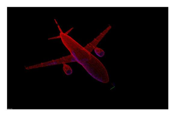
Figure 2.9.: 3d model of an Airbus A320 that was used for matching scans acquired for pose estimation in the aircraft reference frame (red = model points / blue = scanned points)
