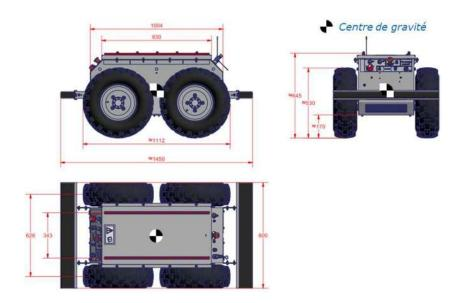
Figure A.4.: Aircobot Dimensions
