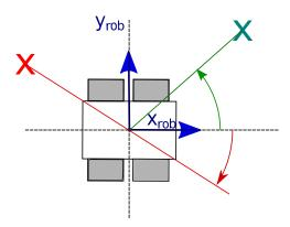
Figure 2.15.: Aligning first with a target "in front" and "behind" the robot
