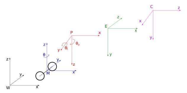
Figure A.1.: Robot coordinate system for the front cameras
