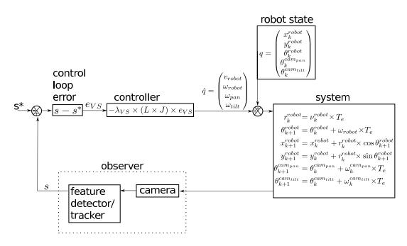
Figure 3.4.: Control loop of an Image-based visual servoing example
