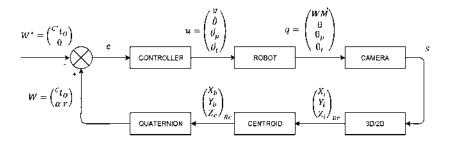
Figure 3.10.: Block diagram for the PBVS approach
