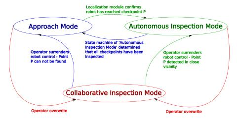
Figure 2.21.: A general overview of the high level state machine of Air-Cobot
