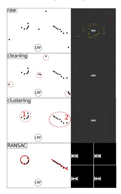
Figure 2.3.: Obstacle detection step by step
