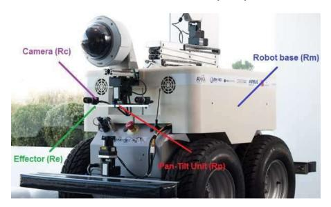
Figure 3.1.: Air-Cobot and the associated frames [Demissy et al., 2016]
