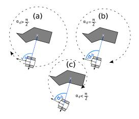
Figure 4.5.: Three schematics of spiral obstacle avoidance patterns
