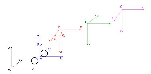
Figure 3.2.: Robot coordinate system for the front cameras [Demissy et al., 2016]
