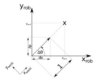
Figure 2.13.: Basics of the mobile base angular velocity  $\omega$  calculation.
