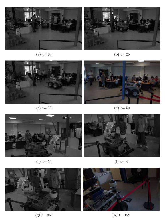
Figure 3.28.: Extract of video sequence showing the systems capability to perform a combination of IBVS-PBVS-Metric based navigation
