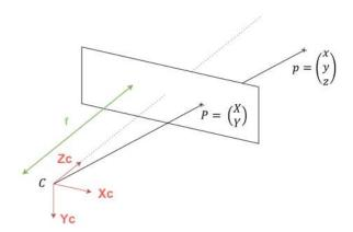
Figure 3.3.: Projection in the image-plane frame
