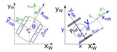
Figure 4.10.: Real life robot model with application point for control inputs
