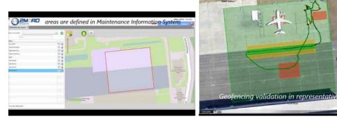
(a) Geo-fencing software interface provided by (b) Overlay of the robots trajectory in a map  $2\mathrm{MORO}$
