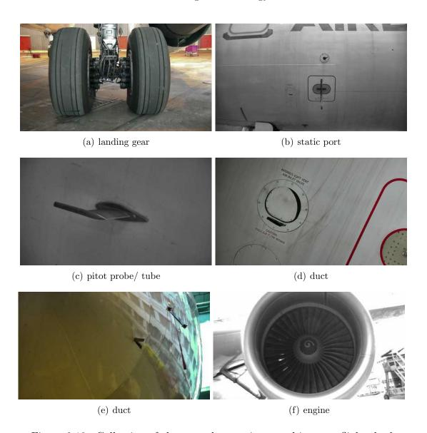
Figure 2.19.: Collection of elements that are inspected in a pre-flight check
