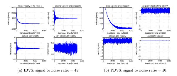
Figure 3.20.: Evolution of velocities in a noisy simulation
