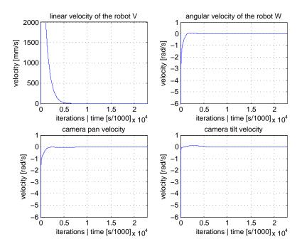
Figure 3.15.: Evolution of velocities in a PBVS simulation
