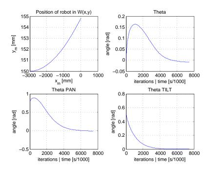
Figure 3.7.: Robot path, orientation and camera state in a IBVS simulation
