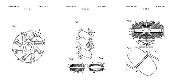
Figure 5.1.: Sketch and cross section of the Mecanum wheel [Ilon, 1975]
