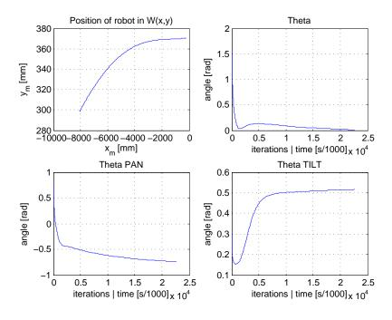
Figure 3.13.: Robot path, orientation and camera state in a PBVS simulation
