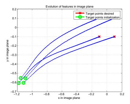
Figure 3.6.: Evolution of features in an IBVS simulation
