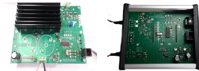
Figure 5.9 Power electronics developed in the LAAS On the left - 1kW bidirectional DC/DC converter, On the right – Control board of the power converter
