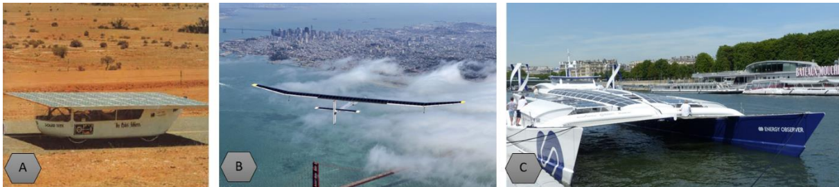
Figure 2.24 Projects of vehicles powered by PV solar systems – A) Quiet Achiever, B) Solar Impulse, C) Energy Observer
