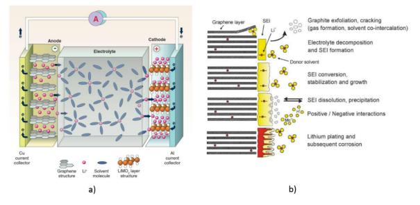
Figure 3.8 Lithium ion battery a) whole cell principle [93] and b) SEI at the anode [91]
