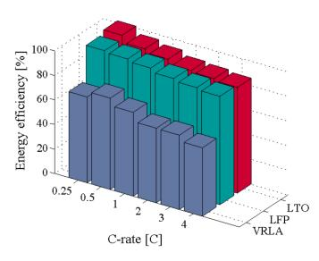
Figure 3.16 Energy efficiency at 25°C under various C-rates [101]
