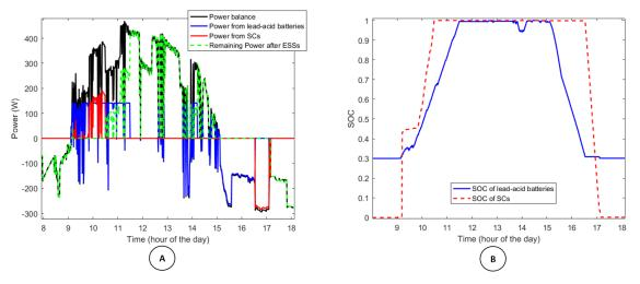
Figure 4. 8 One day of simulation – A) Power profiles, B) SOC profiles
