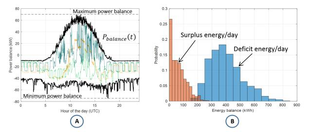
Figure 4.10 ADREAM PV building, A) Minimum and maximum power balance based on a 3-year data set, B) Probabilistic analysis of surplus and deficit energy per day
