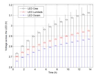
Figure Appendix 4.3 Voltage across each LED for different forward currents
