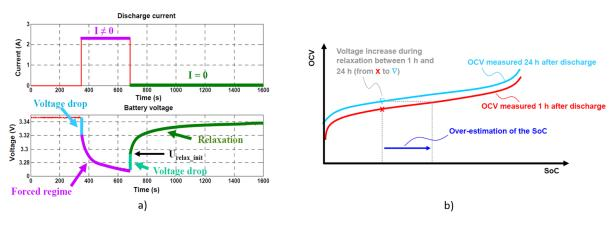
Figure 3.17 a) Voltage relaxation of a lithium-ion battery after a discharge, b) SOC estimation after different relaxation times [107]
