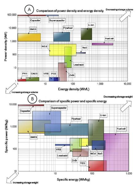
Figure 3.2 Weight and volume characteristics of different ESSs [82]
