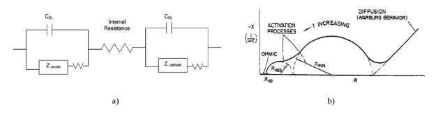
Figure Appendix 3.10 Electrochemical cell modelling by ElS a) Typical equivalent circuit, b) Impedance spectrum in a Nyquist plot [120]
