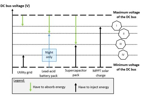
Figure 5.10 Voltage levels and operating modes of the ESSs in the MG
