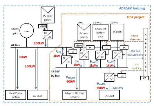
Figure 5.8 Architectures of the developed OPA microgrid and the ADREAM building of the LAAS-CNRS
