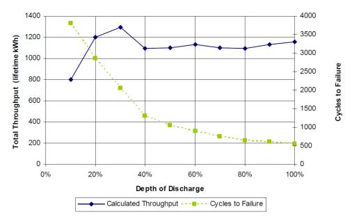
Figure 3.20 Lifetime model of a 2.1 kWh flooded flat plate battery [109]
