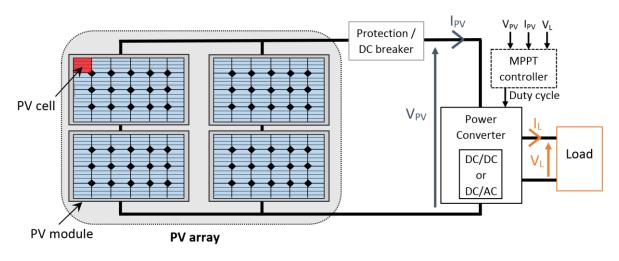
Figure 2.19 Typical PV system feeding a load (AC or DC)
