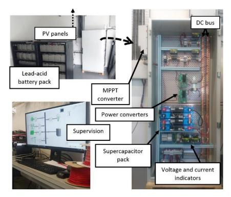
Figure 5.12 OPA experimental setup
