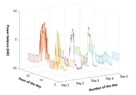
Figure 2.27 Example of power balance of the ADREAM building during 5 days of December 2016
