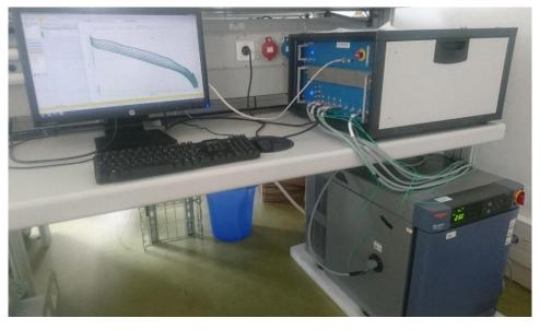
Figure 3.22 Experimental setup for cycling batteries
