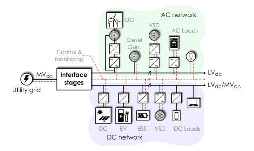
Figure 2.18 Typical hybrid microgrid configuration [44]
