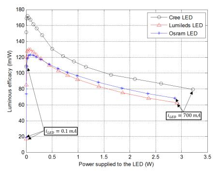
Figure Appendix 4.1 Luminous efficacy vs. Power for three different LEDs
