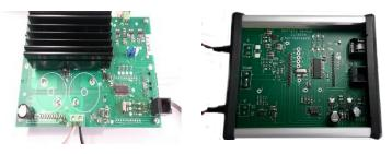
Figure 5.9 Power electronics developed in the LAAS On the left - 1kW bidirectional DC/DC converter, On the right – Control board of the power converter
