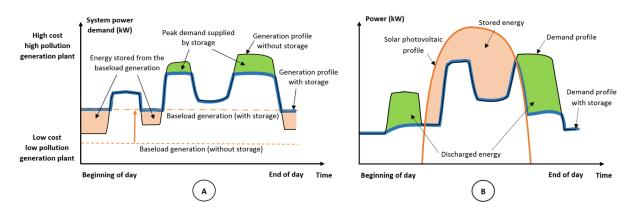
Figure 2.28 Typical use cases of ESS, A) Peak shaving and load levelling, B) Integration of renewable sources
