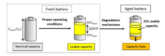
Figure 4.12 Capacity fading of a battery due to ageing
