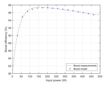
Figure 4.6 Efficiency of a bidirectional DC/DC boost converter for different input power
