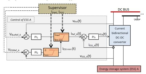
Figure 5.11 Cascade regulation implemented in every power converter of the MG
