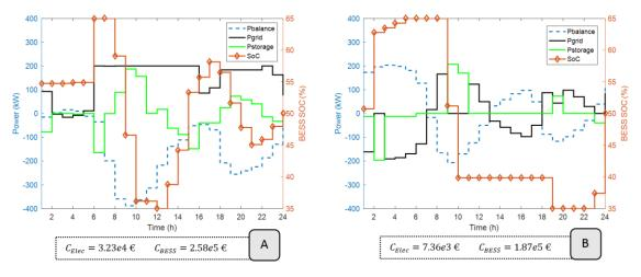
Figure 5.6 MG scheduling for a 1.5 MWh BESS A) Median profile, B) Mean profile
