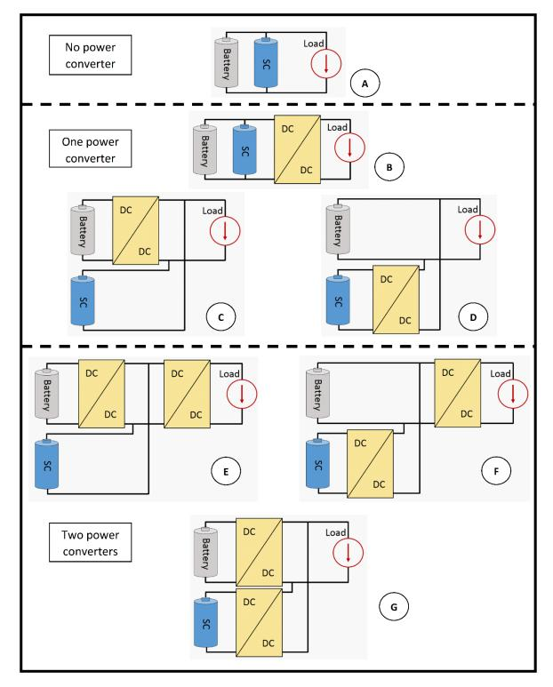
Figure 4.3 Some hybrid topologies of ESSs adapted to DC MGs
