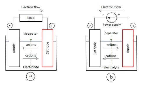
Figure 3.3 Operation of a cell during a) charge and b) discharge.
