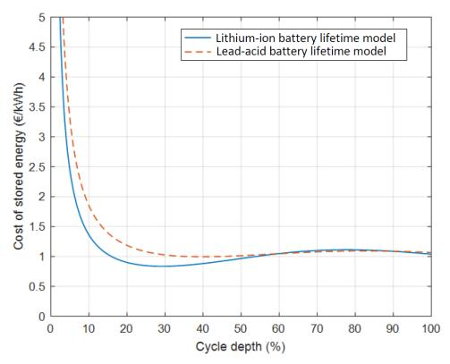
Figure 4.14 Cost of stored energy for different cycle depths and lifetime models
