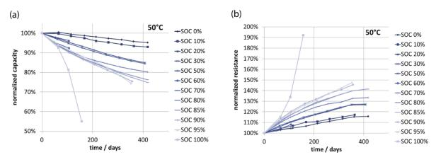
Figure 3.18 Calendar lifetime of lithium-ion batteries at 50°C, a) effect on nominal capacity, b) effect on internal resistance [112]
