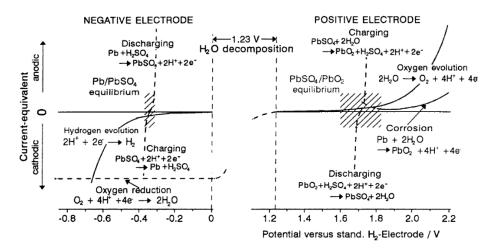
Figure 3.6 Reactions occurring in lead-acid batteries for different electrode potentials [88]
