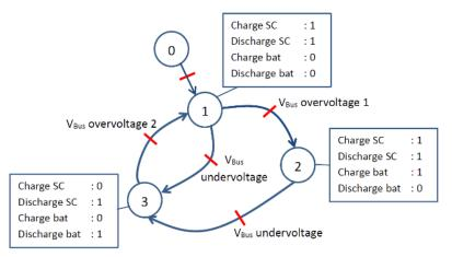
Figure 5. 14 State diagram describing the energy management of ESSs in the MG
