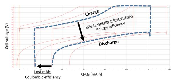
Figure 3.15 Energy and coulombic efficiencies of a Yuasa lead-acid battery
