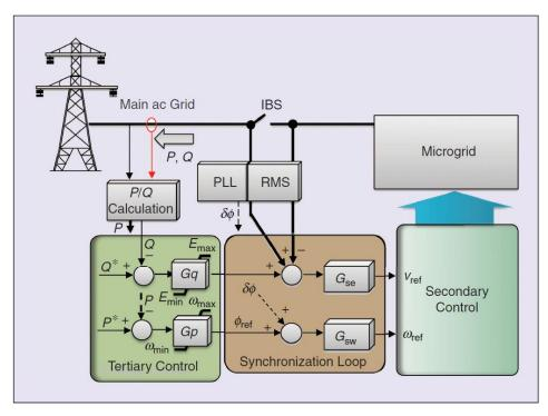
Figure 5.1 Three-level hierarchical control with synchronization control loop [179]
