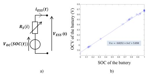
Figure 3.24 a) Simplified model describing an ESS, b) OCV vs. SOC of a lead-acid battery
