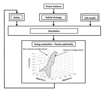
Figure 4.7 Multi-objective sizing methodology of a hybrid ESS
