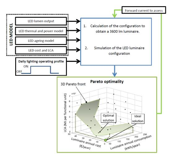
Figure 4.16 Multi-objective methodology developed for LED sizing
