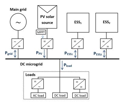
Figure 4.4 Topology of the PV microgrid with two ESSs
