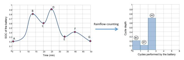
Figure 3.21 Rainflow counting example on an arbitrary SOC time series
