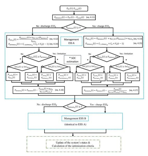
Figure 4.5 Algorithm of ESS management
