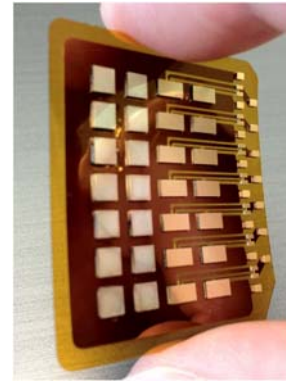
Figure 24 : illustration de l'approche power overlay [21]
