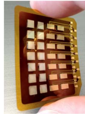
Figure 24 : illustration de l'approche power overlay [21]
