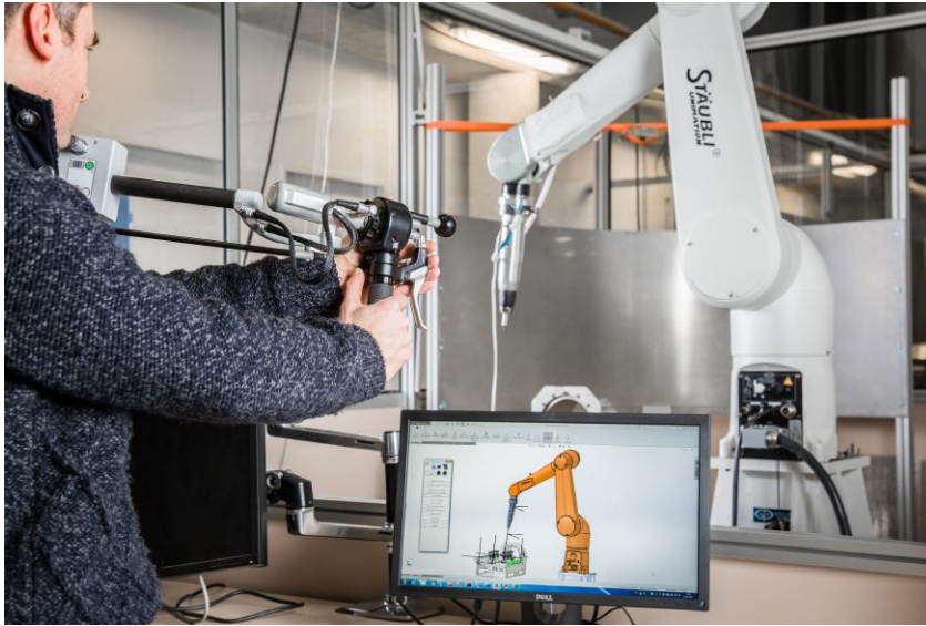
Figure 1.17: Teleoperation of a Staubli robot via a Virtuose 6D haptic device.
