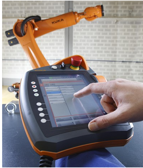
Figure 1.15: Teach-pendant programming interface (smartPAD) for a Kuka robot.
