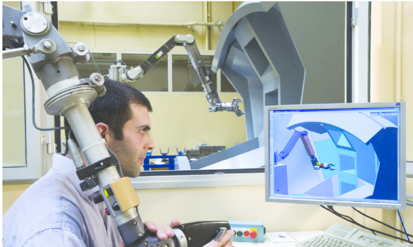
Figure 1.19: In [David 2014] virtual guides are created on the fly into a physical engine, using linear interpolations. Since the guides are not programmed into the real robot controller, slight variations in their respective positions are possible. Also, in the context of co-manipulation tasks it would be more natural to program virtual guides in the real workspace rather than in a simulated one. This is one of the advantages of the hands on approach compared to the teleoperation.
