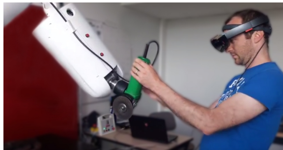
(b) Microsoft HoloLens AR headset, used by our team for the comanipulation of an ISybot robot.
