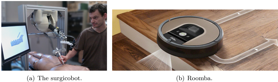
Figure 1.4: Examples of recent innovative human-robot interfaces and sensors. a) The Surgicobot robot. Designed for milling assistance, especially in orthopedic surgery. It was developed by HAPTION (Laval, France) as part of the Surgicobot project (ANR Tecsan). Image extracted from [Françoise 2013a], where different control strategies for Surgicobot are proposed. b) iRobot Roomba Vacuum service robot. This mobile robot is equipped with a camera that allows it to navigate using VSLAM (Vision Simultaneous Localization and Mapping).
