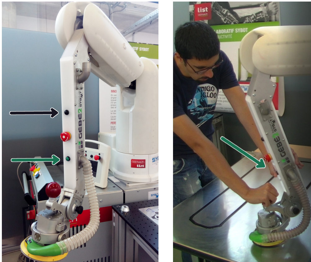
(a) Cobot programming interface. Lower green button is used to record key points. Upper black button is used to end the recording and activate the virtual guide.
