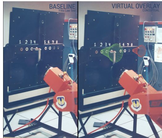
Figure 6.2: Augmented reality application on telerobotic control of Fitt's Law peg-board task [Rosenberg 1993]. Image by GardenM - Own work, CC BY-SA 4.0.
