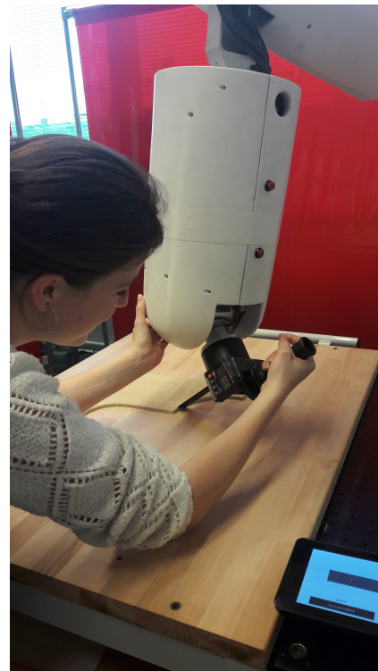
(b) Manipulation by the handle of the tool and the 4 th body of the arm
