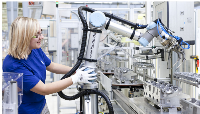
Figure 1.7: Collaborative robot from Universal Robots (UR5) used in Volkswagen's production line - "...While safety is imperative, that's simply the cost of entry into the cobot market now. We believe that being collaborative is just as much being accessible, lowering the automation barrier by placing robots within reach of manufacturers that never thought they would be able to deploy robots." Universal Robots.
