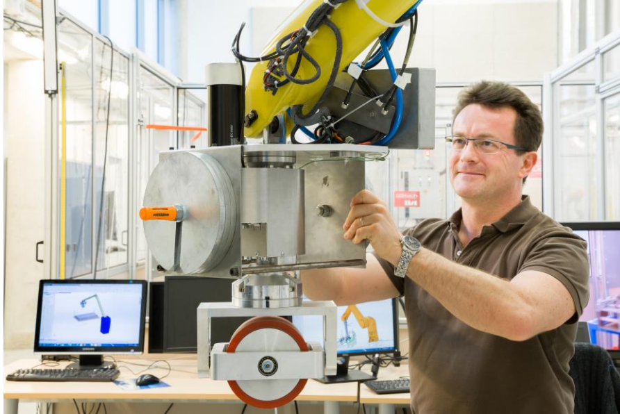
Figure 2.2: Direct manipulation of the Cobomanip cobot designed by CEA-List and Sarrazin to assist the operator during handling operation.
