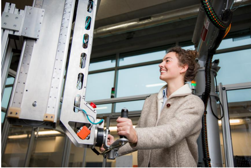
Figure 1.20: Scara cobot conceived by CEA . This image shows an example of hands-on interaction where the user directly manipulates the robot.
