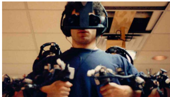
(a) AR interface proposed by [Rosenberg 1993], used in teleoperation tasks.
