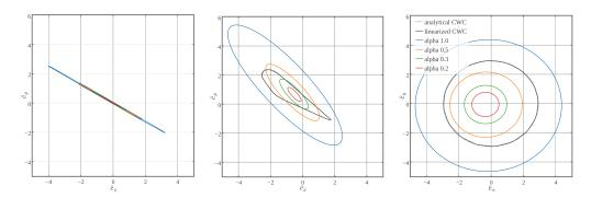
Figure 4.7: Illustration of the contact wrench approximations for scenarios of Fig. 4.5. The exact CWC and its linear approximation closely matches. The outer approximation is obtained with  $\alpha = 1$ , and the inner approximation with  $\alpha = 0.2$ . The approximation  $\alpha = 0.3$  is an efficient trade off.
