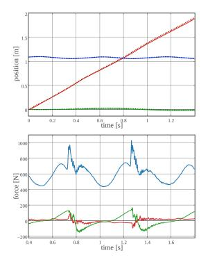
Figure 2.8: CoM position reconstruction for natural walking (red for x, green for y and blue for z). On the left, the reconstructed CoM in plain line and the CoM coming from geometry in dotted line. On the right, the force measurement during a short period.
