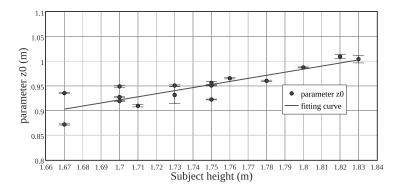
Figure 3.8: Evolution of the mean altitude  $z_0$  according to the subject's size. The standard deviation of this parameter for each subject is very weak (below 2mm). Furthermore, the altitude is strongly correlated to the size of the subjects  $p \leq 0.001$  with a correlation coefficient of 0.87.
