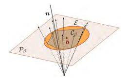
(a) Estimate of the plane direction  $\boldsymbol{n}$  from the collection of rays contained in  $K_c^6$ . Outer ellipsoid  $\mathcal{E}$  estimated from the convex-hull  $\mathcal{C}(\boldsymbol{n},\beta)$  obtained from the ray projection onto the plane  $P(\boldsymbol{n},\beta)$ .
