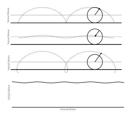
Figure 3.3: Illustration of the three types of cycloid. From top to bottom: normal cycloid, curtate cycloid and prolate cycloid. The last plot corresponds to the CoM trajectory in the sagittal plane. Its shape is very similar to the curtate cycloid.
