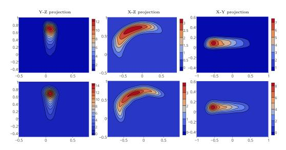
Figure 4.4: Illustration of the probability density distribution of the CoM w.r.t. the right foot frame of TALOS, projected along the three axis X,Y,Z. The first row corresponds to the ground truth distribution estimated through KDE (20000 points). The second row depicts the learned GMM with 4 Gaussian kernels in the mixture. The axes have the same scale than in Fig 4.2.
