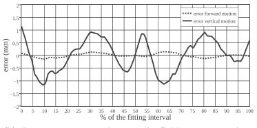
(b) Reconstruction error between the CoM trajectory and its fitting with the proposed model. Over the whole cycle, the reconstruction error remains below 1.5mm and it is mainly contained in the vertical direction.
