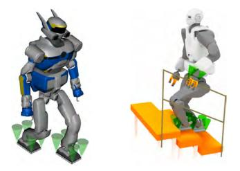
Figure 4.1: Illustration of HRP-2 robot and TALOS robot making contacts with their environment. The green "ice-cream" cones are dispatched on the 4 vertices of the feet, symbolizing the friction cones with friction coefficient of value 0.3.
