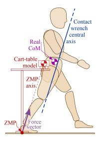
Figure 2.2: Illustration of various notations. A graphic representation of the comparison between the central axis of the contact wrench and the ZMP. The ZMP part is depicted in red and shows the approximation made by the cart table model. The line joining the ZMP to the CoM of the cart-table model is parallel to the contact force vector. The central axis part is shown in blue. It is the line of minimal moment norm, also parallel to the contact force vector.
