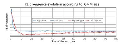
Figure 4.3: Evolution of the KL divergence between the KDE distribution and GMMs of different sizes for the four end-effectors of the HRP-2 robot.
