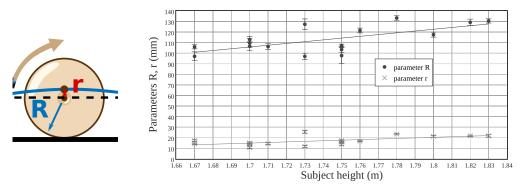
Figure 3.7: On left, the scheme of the wheel with the notations of the model: R is the radius of the wheel while r is the distance of the point to the wheel center. On right, a scatter plot showing the evolution of the mean radius parameters R and r according to the subject's sizes. The standard deviation of the parameters is low (below 5mm) for all the subjects. It appears that these two parameters are correlated to size of the subjects.
