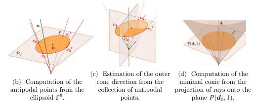
Figure 4.6: Illustration of the procedure to build the outer approximation of the CWC from the collection of rays coming from the linearization of the contact cones.
