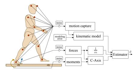
Figure 2.1: Scheme of the merging processus. The problem of merging measurements for CoM reconstruction in the presence of noises and modelling errors.
