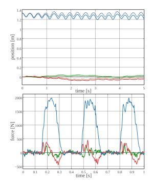
Figure 2.9: CoM reconstruction for running on a treadmill (red for x, green for y and blue for z). On the left, the reconstructed CoM in plain line and the CoM coming from geometry in dotted line. On the right, one second of force measurement
