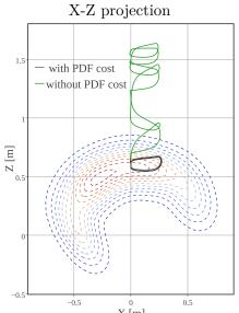
Figure 4.9: Projection of the CoM trajectory inside the right foot frame with and without taking into account the log-pdf term in the cost function. The level set corresponds to the GMM distribution used in our OCP.
