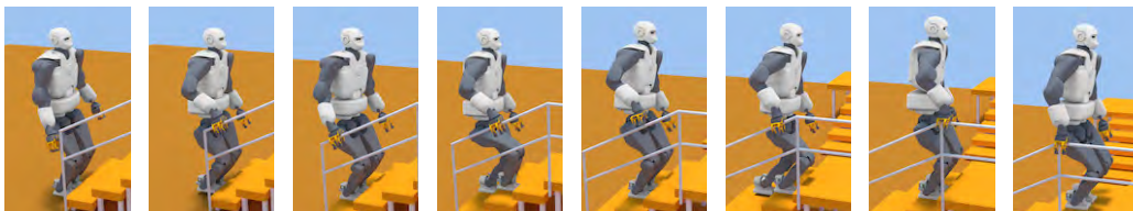
Figure 4.12: Snapshots of the climbing 15-cm high steps motion with handrail by the TALOS robot in simulation.
