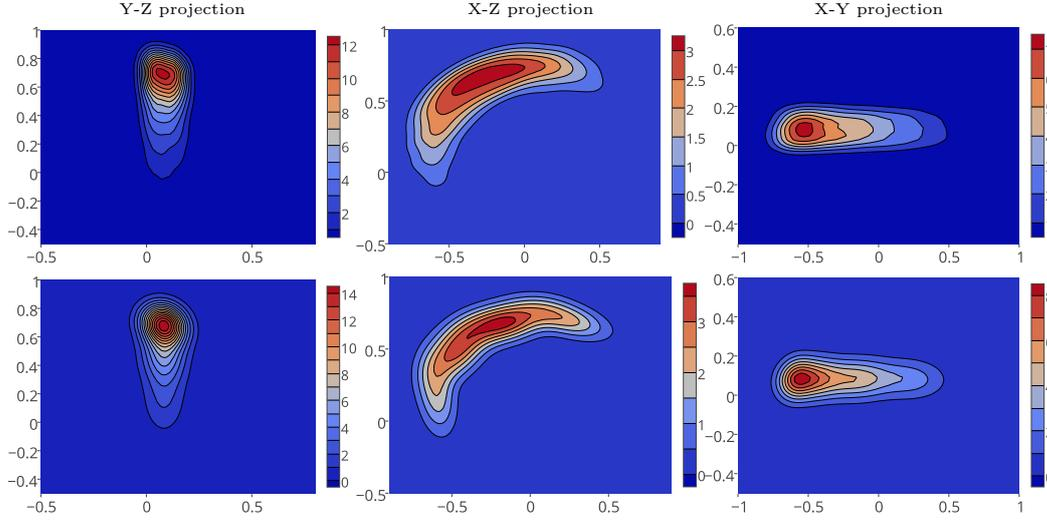
Figure 4.4: Illustration of the probability density distribution of the CoM w.r.t. the right foot frame of TALOS, projected along the three axis X,Y,Z. The first row corresponds to the ground truth distribution estimated through KDE (20000 points). The second row depicts the learned GMM with 4 Gaussian kernels in the mixture. The axes have the same scale than in Fig 4.2.
