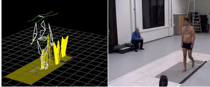
Figure 3.2: Capture of the experiment room during the acquisition session. A male subject was instructed to walk barefoot in straight line at his comfort walking speed on two force platforms. Two force plates are firmly embedded in the floor and allows the reconstruction of the segmentation of the walking pattern.
