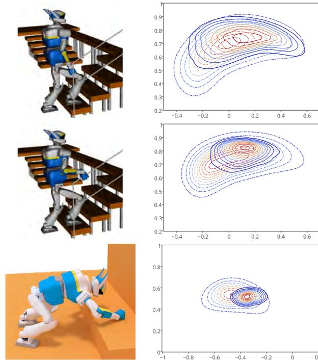
Figure 4.5: Checking of the CoM independence hypothesis for various scenarios. (Left) contact configurations and (right) corresponding level sets of the CoM occupancy measures, with ground truth in solid lines and approximations in dashed lines. On the first row, the robot makes two contacts with the stairs while on the second one, the robot is also handling the handrail. On the last row, the robot is making 4 contacts.
