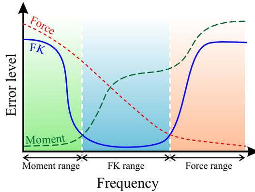
Figure 2.3: **Illustration of the intuition on spectral distribution.** A sketch representation of the spectral distribution of errors that would emerge from the naive reconstruction of CoM trajectory if we use only one signal (Geometry, Forces and projection of the CoM from Geometry onto the Contact Wrench Central Axis). The signal with the lowest error is then selected at each frequency bandwidth to constitute minimal-error fusion of these signals.
