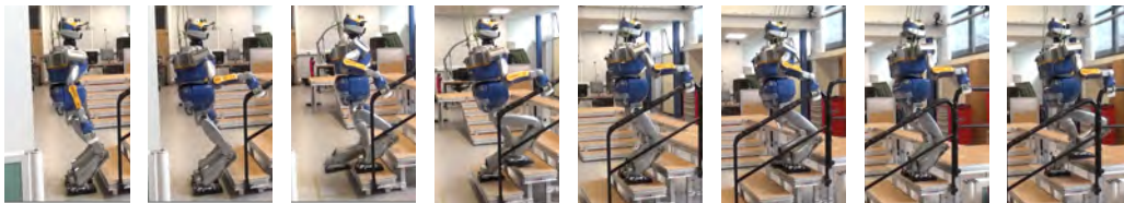
Figure 4.11: Snapshots of the climbing up 15-cm high steps motion with the HRP-2 using the handrail.
