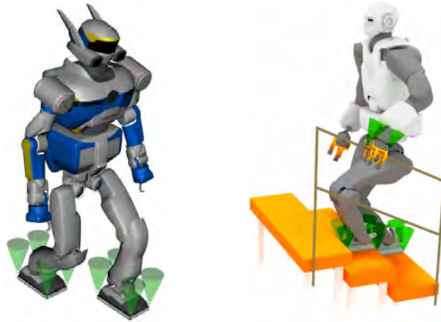
Figure 4.1: Illustration of HRP-2 robot and TALOS robot making contacts with their environment. The green “ice-cream” cones are dispatched on the 4 vertices of the feet, symbolizing the friction cones with friction coefficient of value 0.3.
