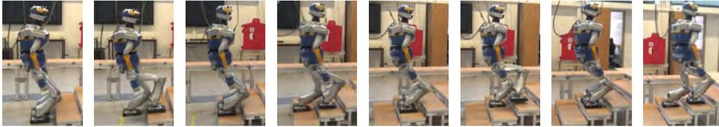
Figure 4.10: Snapshots of the climbing up 10-cm high steps motion with the HRP-2 robot.
