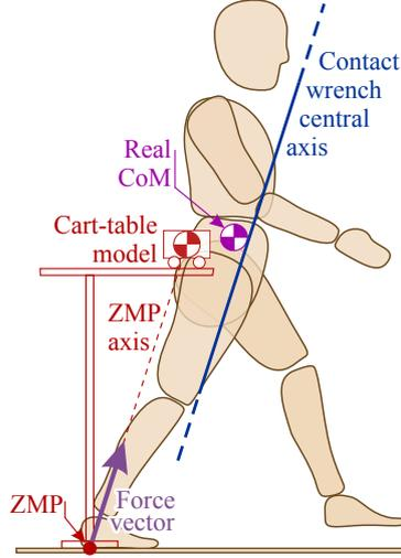
Figure 2.2: **Illustration of various notations.** A graphic representation of the comparison between the central axis of the contact wrench and the ZMP. The ZMP part is depicted in red and shows the approximation made by the cart table model. The line joining the ZMP to the CoM of the cart-table model is parallel to the contact force vector. The central axis part is shown in blue. It is the line of minimal moment norm, also parallel to the contact force vector.
