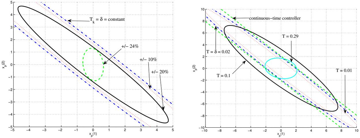
(a) Influence of  $\mathcal{T}_1$ , and  $\mathcal{T}_2$  with  $\mathcal{T}_1 = \delta - \mu$  and  $\mathcal{T}_2 = \delta + \mu$  on the ellipsoidal regions of stability in the system plane ( $x_c = 0$ ) considering  $\delta = 0.02$  and the following cases:  $\mu = 0$  (dashed-dotted line),  $\mu = 10\% \delta$  (dotted line),  $\mu = 20\% \delta$  (solid line) and  $\mu = 24\% \delta$  (dashed green line).
