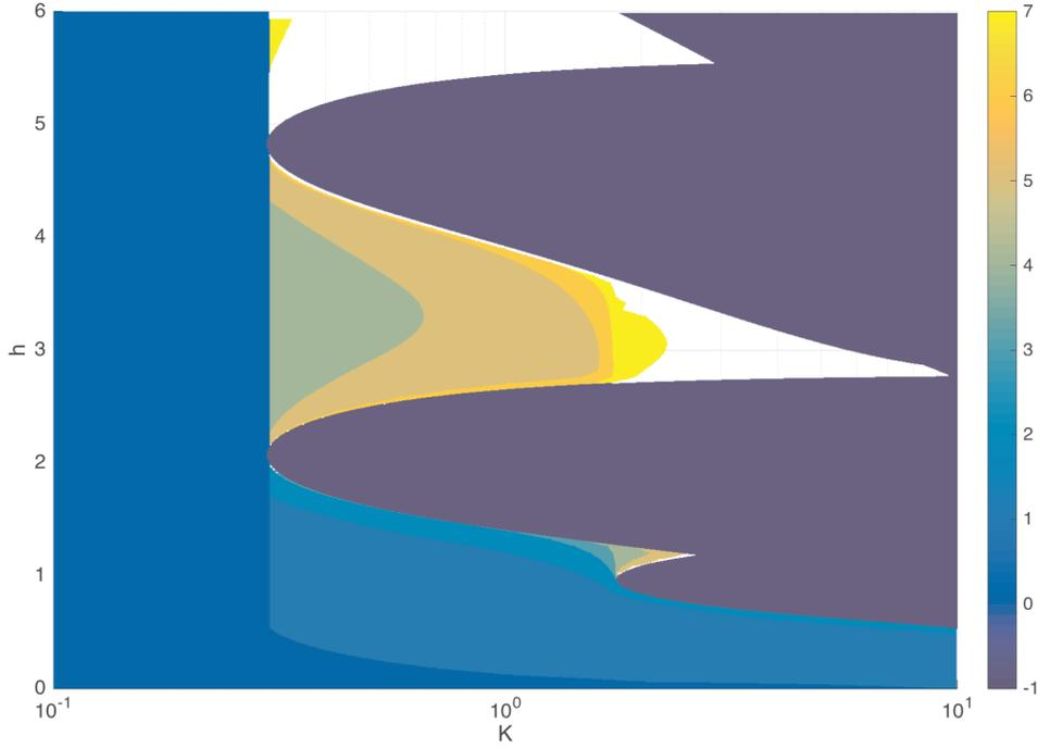
Figure 2.4: Stability region in the plan  $(K, h)$ , obtained using Theorem 2.3 for  $N = 0, \dots, 7$ . The instable area, computed through a frequency analysis corresponds to the dark area, which is depicted with the color associated to  $N = -1$
