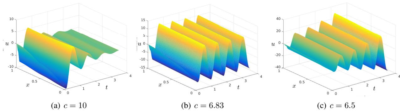
Figure 1.8: Chart of  $u$  for system composed of the coupling of an ODE and the wave PDE, characterized by the wave speed  $c$  with the parameters:  $u^0(x) = (\cos(\pi x) + 1) \frac{KX_0}{2}$ ,  $X(0) = [1 \ 1]^T$ ,  $v^0(x) = 0$  and  $c_0 = 0.15$  for 3 values of  $c$ , presented in [24].
