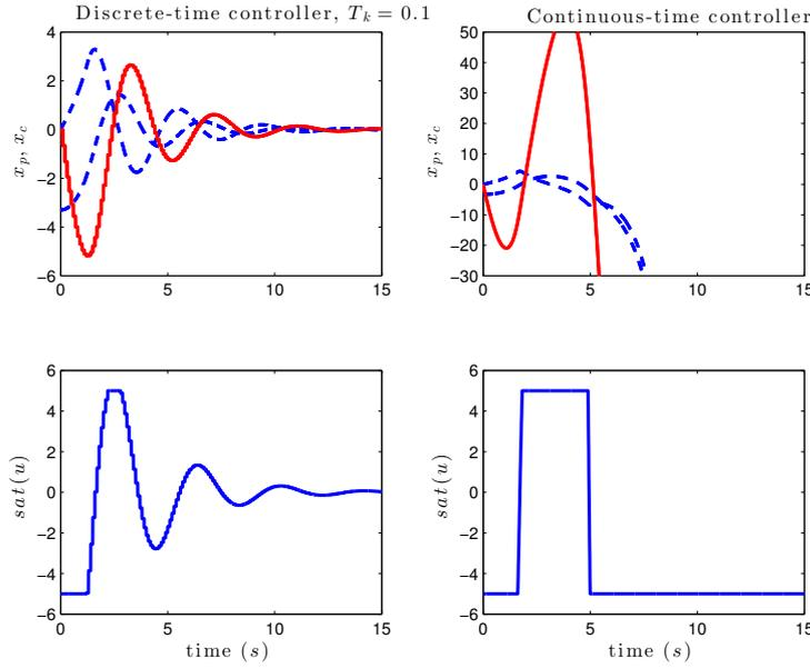
Figure 3.6: Time response of the closed-loop system. Left-hand side: with discretized controller given by matrices in (3.43) and implemented with a periodic sampling  $T = 0.1$ . Right-hand side: with the continuous-time controller given by matrices in (3.42).
