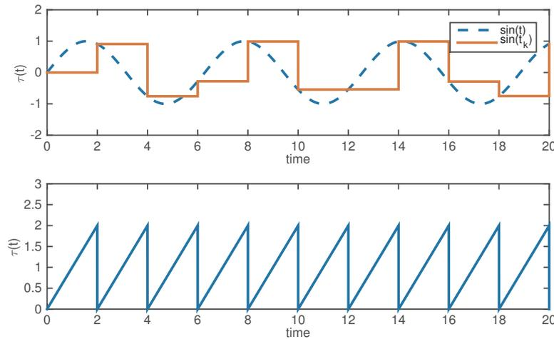
Figure 3.2: Illustration of a periodic sampling delay  $\tau(t)$ .
