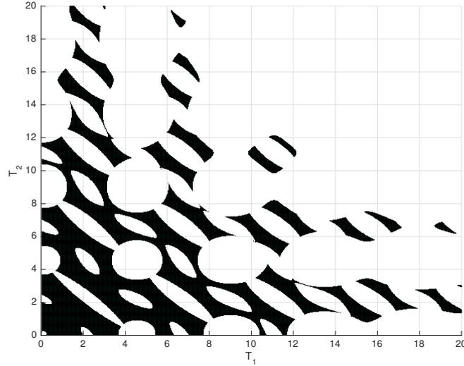
Figure 3.1: Stability region in the plan  $(T_1, T_2)$  of sampled-data system (3.6) with the sampling rule (3.7). The black areas corresponds to stable behaviors of the sampled-data system (3.6).
