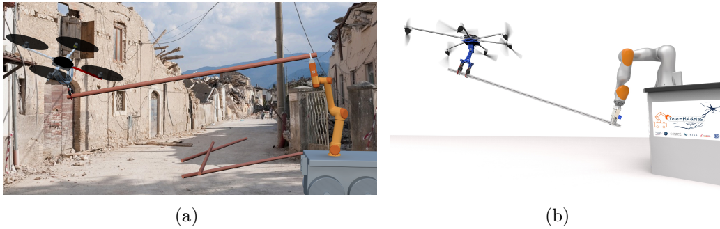
Figure 3.2 – Potential use cases for MAGMaS of different composition. Left (a) in a USAR scenario with a mobile base and an underactuated AR cooperatively cleaning buildings remains. Right (b) in a decommissioning scenario with a fixed ground robot and a multi-directional thrust AR cooperatively manipulating a pipe.
