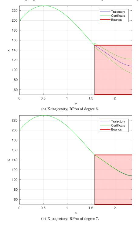
Figure 4.6 – X-coordinate in function of true anomaly for RPAs of degrees 5 and 7.
