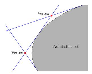
Figure 2.6 – Original admissible set (dashed line) and admissible set obtained after discretization (continuous lines).
