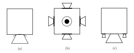
Figure 1.14 – Thruster configurations: (a) p = 2, (b) p = 1 and (c)  $p = \infty$ .
