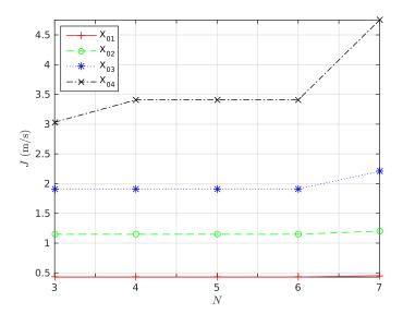
Figure 3.13 – Impact of number of impulses on fuel consumption.
