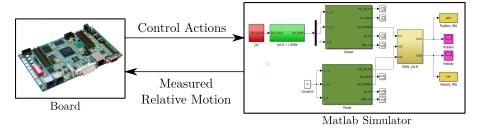
Figure 3.6 – Processor-in-the-loop environment: network connection between board and simulator via user datagram protocol.
