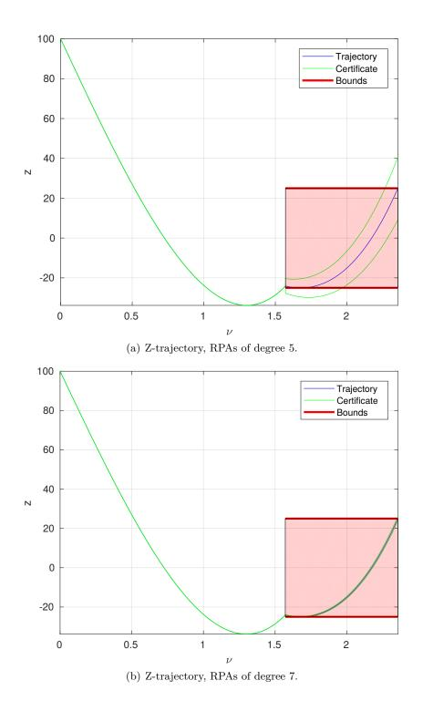
Figure 4.7 – Z-coordinate in function of true anomaly for RPAs of degrees 5 and 7.
