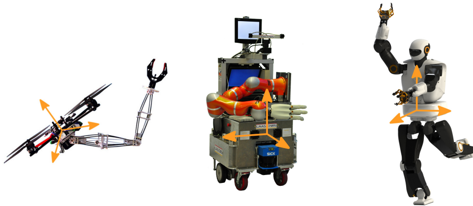
Figure 7.4: Three different multi-joint mobile robots at LAAS: the flying manipulator Aeroarm (left), the mobile manipulator Jido (center), and the humanoid robot Talos (right). The usual choices for their root frame placement are displayed.
