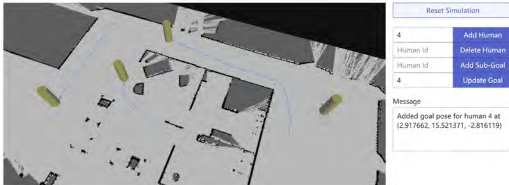
Figure 3.5 – A human motion simulator that can simulate 2D motion of multiple humans. Cylinders represent current human position and associated radius. The blue lines show the paths that each simulated person is following. The panel on the right side allows to manipulate number of simulated persons and their goal positions.
