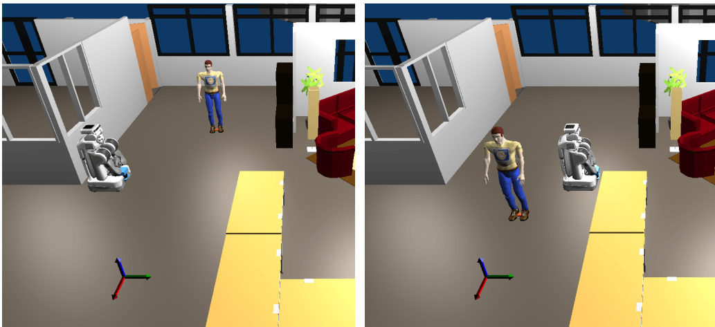
Figure 3.4 – A human-robot path crossing scenario created in MORSE simulator. The figure on the left shows the situation a few seconds before the situation of figure on the right. The robot and human had crossed their paths during this time.
