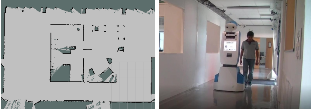
Figure 3.2 – Experiment area with motion capture system to detect human positions and velocities. Figure on the left shows an image of a person being guided by the robot, the robot tracks the helmet that the person is wearing with the motion capture cameras Figure on the right shows map of an area where we have installed the motion capture system.
