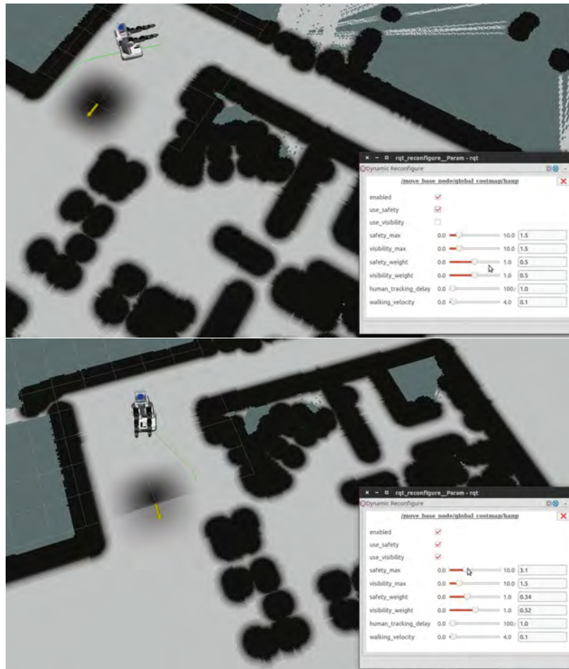
Figure 3.1 – Proxemics costs for path planning (in shades of black to white, darker shades denote higher costs) and generated path (green). Arrow (yellow) denote tracked position of a person.
