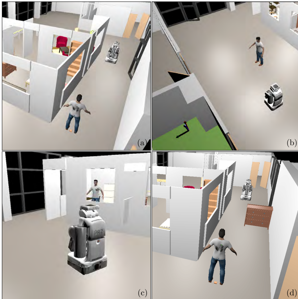
Figure 4.11 – Canonical human-robot path crossing situations. (a) Human and robot crossing each other’s path on a corridor. (b) 90^\circ path crossing situation. (c) Human coming out of a room where robot needs to go, they cross each other at the door. (d) Similar to situation 4.11a, however the drawer is blocking the corridor in such a way that only one person (or robot) can pass next to the drawer at a time.
