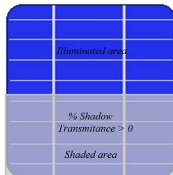
Fig. 3.6 Partially shaded PV cell
