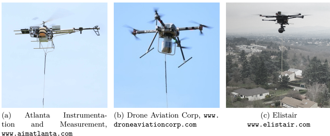
Figure 4.1 – Examples of companies proposing tethered aerial robots for long flight time operations.
