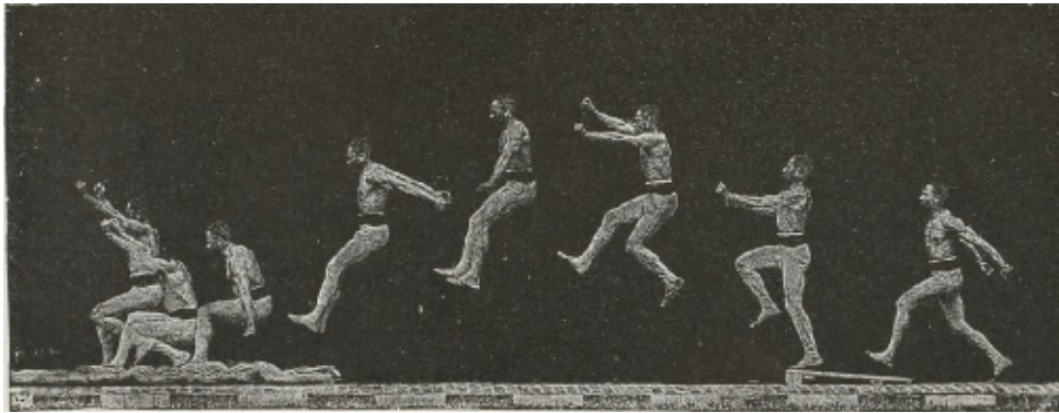
Figure 1.2: Successive phases of a jump motion for kinematics study. The image was taken at 5 [Hz] using chrono-photography on fix plate. The photo appears in the book "Le MOUVEMENT" by Étienne-Jules Marey, 1984.
