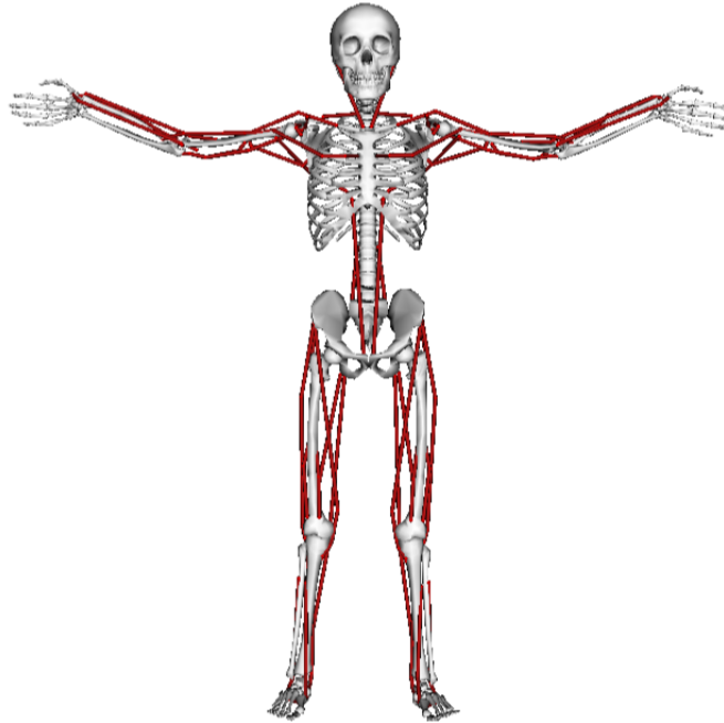
Figure 2.12: Musculoskeletal model. The visual elements are based on the running model of Hammer [Hamner 2010].
