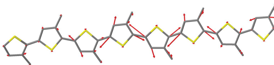
Figure 4. Representation of the atomic displacements involved in the collective stretching \mathcal{A} mode.
