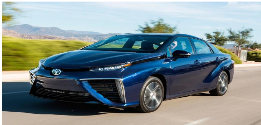
Figure 54: 2015 - TOYOTA Mirai, with a 114 kW fuel cell (155 horses), and a 1.6 kWh Ni-Mh battery.
