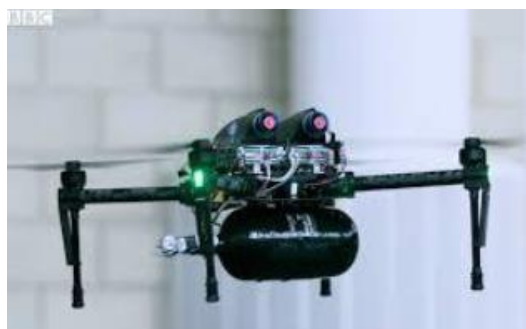
Figure 57: Hydrogen drone designed by the company Intelligent Energy using fuel cells.
