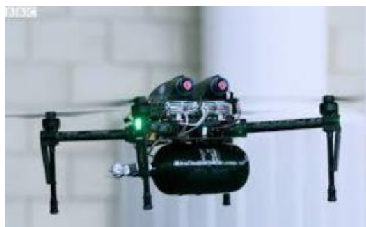
Figure 57: Hydrogen drone designed by the company Intelligent Energy using fuel cells.
