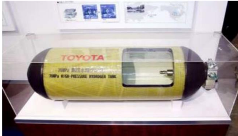
Figure 59: Composite Hydrogen reservoir from the brand Toyota
