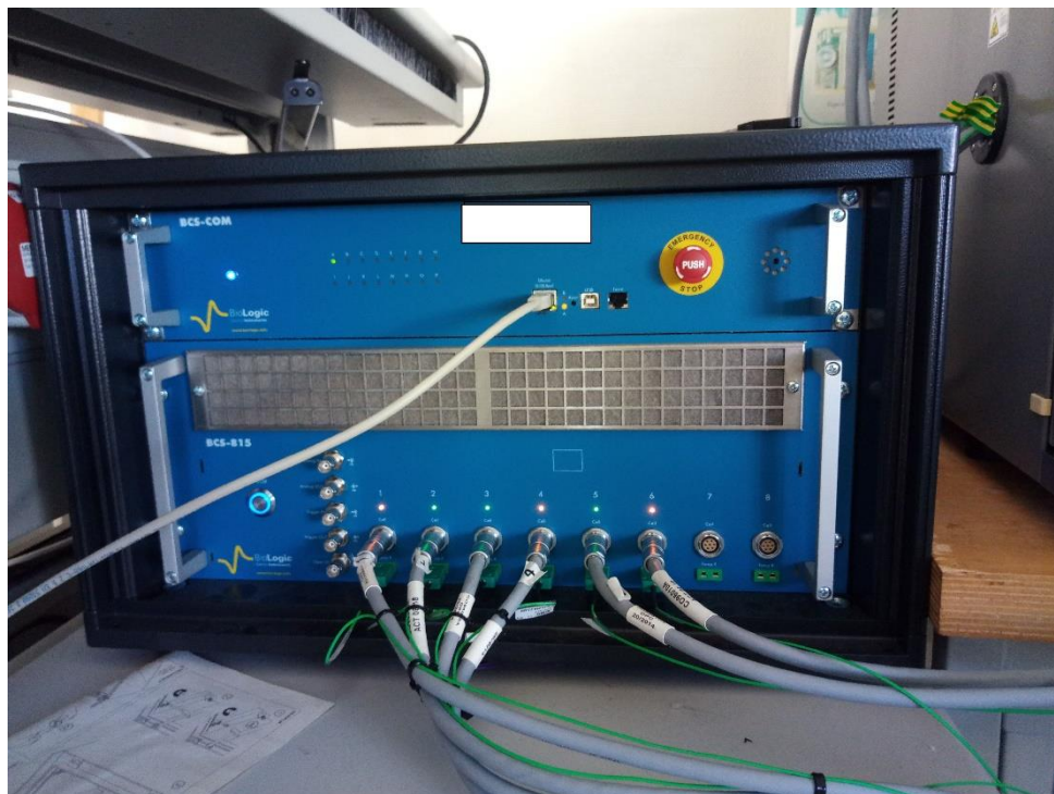
Figure 31: BCS-815 battery cycler from Bio-Logic installed in the laboratory room of the ADREAM platform
