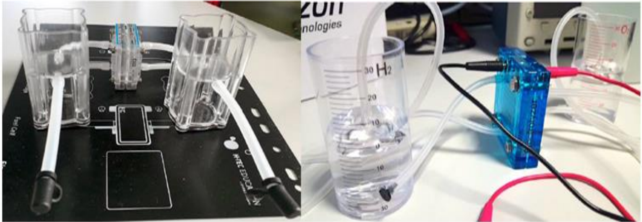
Figure 74: The two electrolyzers connected to graduated reservoirs via plastic tubes, experimental setup
