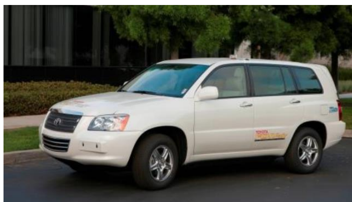
Figure 52: Toyota - FCHV-adv model 2009. Advanced fuel cell vehicle with four high pressure hydrogen tanks at up to 700 bar, precursor to the more known Toyota Mirai.
