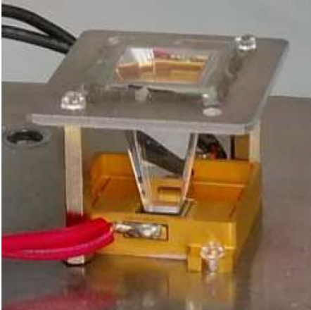
Figure 87: Triple junction cell with solar prism.
