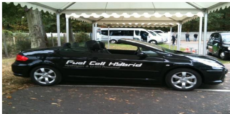
Figure 51: 2009 - Peugeot 307 cc FiSyPAC hybrid electrical prototype, equipped with JCS Li-ion batteries and a CEA-PSA 20kWe fuel cell stack as a « range extender »
