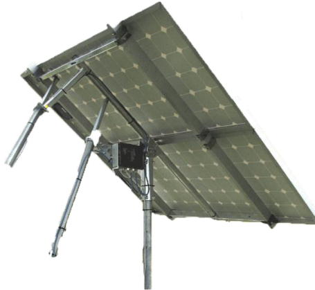
Figure 89: Two-axis solar tracker installed in the LAAS laboratory
