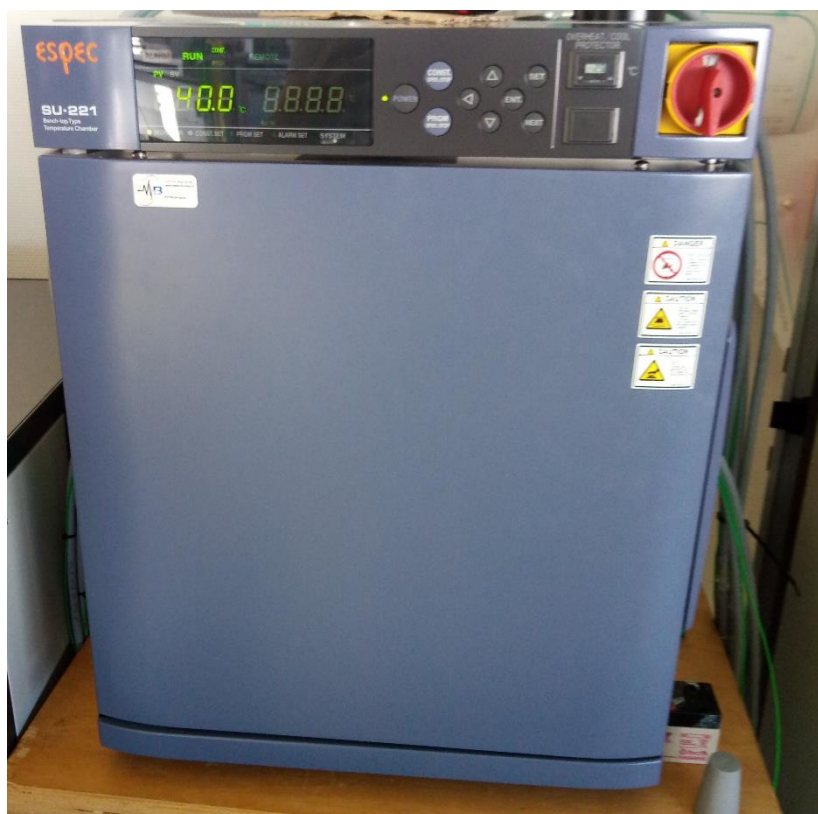
Figure 32: Thermal enclosure used with the BCS-815 for temperature control during battery tests
