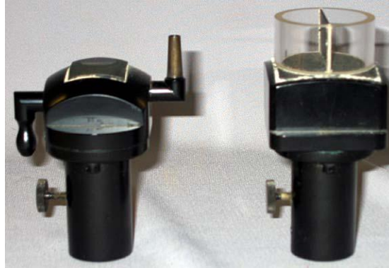
Figure 1.7. Metal water-jacket to control temperature in the Pulfrich refractometer [68].
