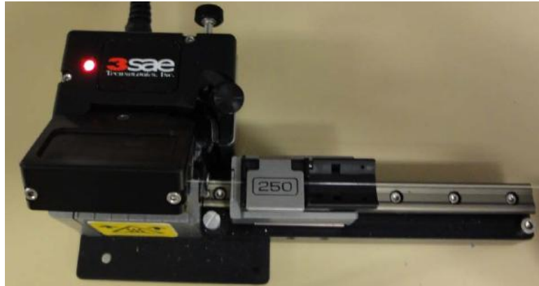
Figure 2.7. Thermal stripper for removing MMF cladding as well as fiber coating.
