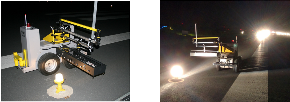
Figure 2.1: Sterela robot measuring runway lamps
