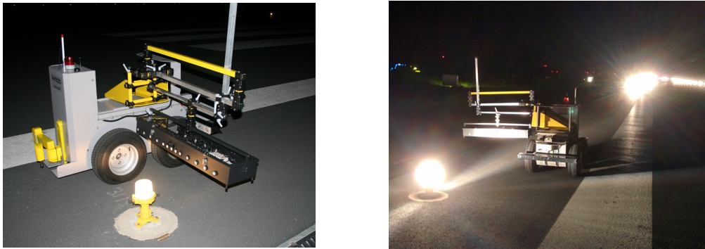
Figure 2.1: Sterela robot measuring runway lamps
