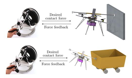
Figure 3.5: The scenarios of aerial teleoperation for physical interaction with contact considered in (Gioioso et al. 2015). Top: docking to a surface. Bottom: pushing a cart.
