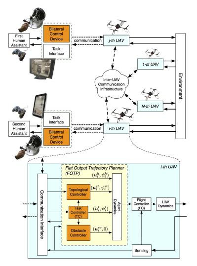
Figure 2.8: Architecture and overall framework of the shared control of multiple mobile robots.
