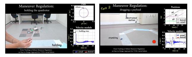
Figure 2.17: Experiments with a cm-scale aerial robot showing the robustness of the maneuver regulation approach (**Spedicato**, **Franchi**, and Notarstefano 2016) when the aerial robot is subject to unexpected external disturbances such as 'holding' (left) and 'unknown payload dragging' (right).
