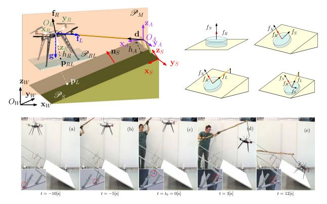
Figure 2.19: An experiment showing the use of the developed tethered control and planning methodology to robustly land on a sloped surface (perching).
