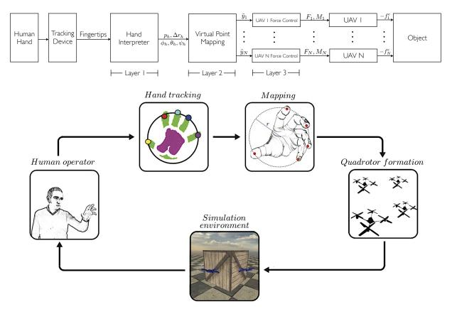
Figure 3.11: Block diagrams of the flying hand collaboration concept. Each aerial robot acts as a single finger to grasp an object and the is teleoperated by a human hand through the use of a suitable abstraction layer (**Gioioso** et al. 2014a).
