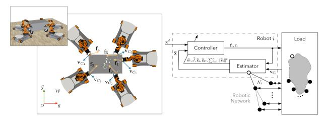
Figure 2.22: Fully-decentralized cooperative manipulation with unknown load parameters, unknown grasping parameters, and unknown load state.
