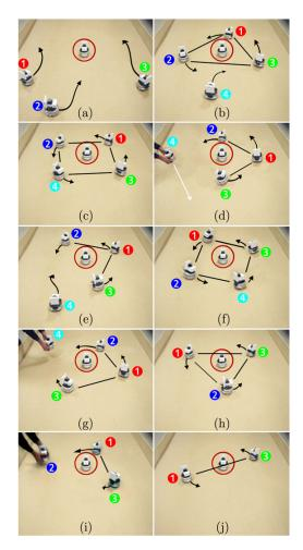
Figure 2.6: Experiments of the decentralized encirclement control with moving target and kidnapping.
