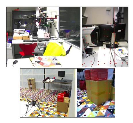
Figure 2.12: Semi-autonomous quadrotor that can be bilaterally teleoperated (i.e., with haptic feedback) by a remote user. The employed sensors are only the onboard RGB-D camera and IMU (no external motion capture is used).
