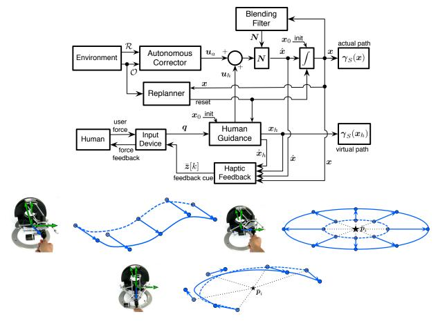
Figure 3.3: Top: block diagram of a feedback-force human-robot collaboration scheme with relatively long time horizon in the operator reference.
