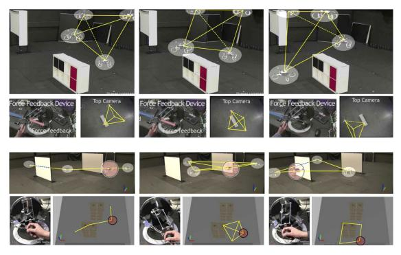
Figure 2.10: Experiments of shared control of multiple mobile robots. Fixed Topology versus time-varying topology case.
