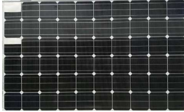
Figure 2.28 Test for shadow on a module Tenesol 2200 with shadows on February 9th, 2018
