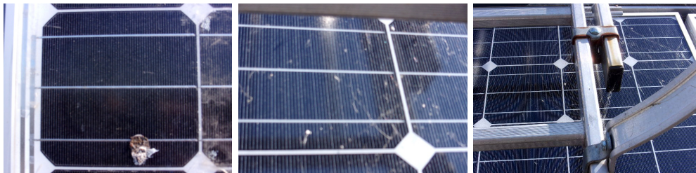
Figure 1.17 Example of other types of obstacles generating shadow problems on PV modules (bird droppings, cobwebs, and fixed obstacles such as stairs)
