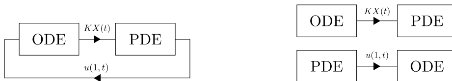
(a) Coupled system (3.1) with B \neq 0 and K \neq 0 (b) Cascaded system (3.1) with B = 0 (top) and K = 0 (bottom)
