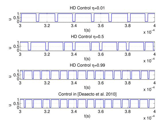
Figure 4.6: Zoom of u in the boost converter.
