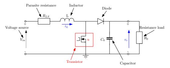
Figure 2.2: Boost converter circuit.
