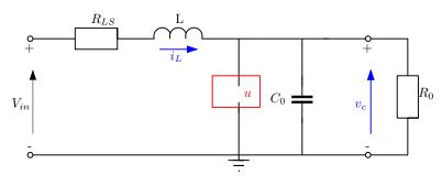
Figure 2.4: Boost converter circuit (OFF).
