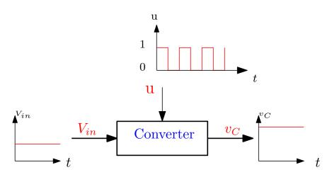
Figure 2.1: Illustration of the boost converter objective.
