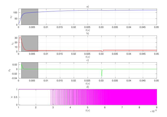
Figure 4.9: Evolutions for  $\gamma = 50 \cdot 10^{-4}$  of the voltage and current in a) and b) resp.,  $\ddot{x}_2$  in c) and, zoom of u in d)
