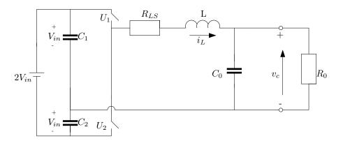
Figure 2.7: Half-bridge inverter.
