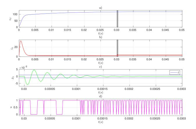
Figure 4.11: Evolutions for  $\gamma = 1$  of the voltage and current in a) and b) resp., and zoom of  $\breve{x}_2$  and u in c) and d) resp.
