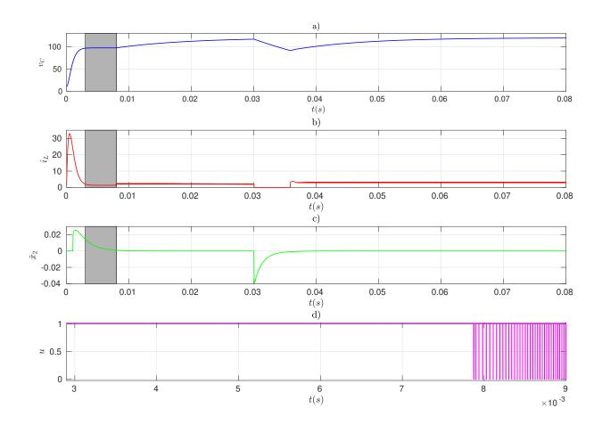
Figure 4.8: Evolutions for  $\gamma = 5 \cdot 10^{-4}$  of the voltage and current in a) and b) resp.,  $\ddot{x}_2$  in c) and, zoom of u in d).
