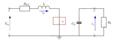
Figure 2.3: Boost converter circuit (ON).
