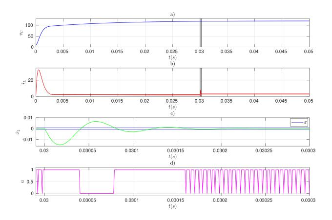
Figure 4.10: Evolutions for  $\gamma = 0.1$  of the voltage and current in a) and b) resp., and zoom of  $\breve{x}_2$  and u in c) and d) resp.
