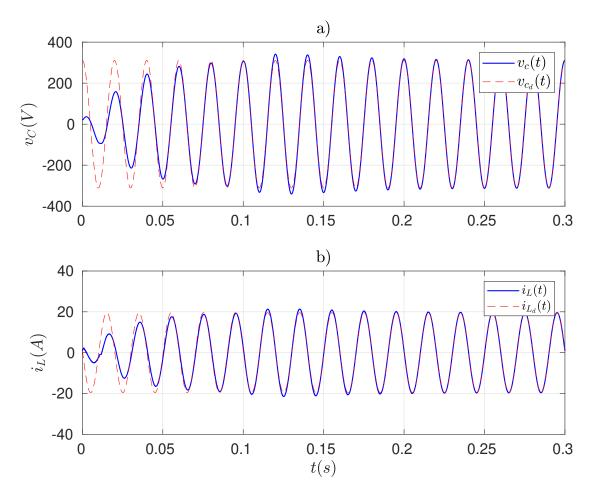
Figure 5.2: Evolution of voltage and current for  $\alpha = 400$ .
