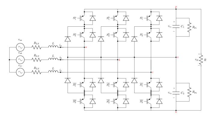
Figure 2.5: Three-phase three-level neutral point clamped (NPC) rectifier.
