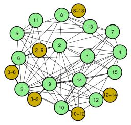
(b) Computed virtual map —virtual sensors indicated in yellow are labelled with intersecting physical sensors label set.
