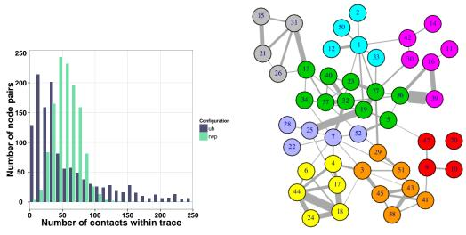
(a) Weight distributions of the wireless contact graphs generated from the (user-based, ub) collected data, and from the (random waypoint, rwp) model.
