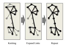
Figure 14: Algorithm DICT first discovers and reserves sequences of highly connected parts of the host graph. Then, less connected parts are discovered by edge expansion and then the process is repeated until no additional nodes and edges can be found.
