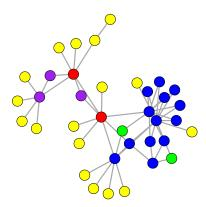
Figure 16: Representation of the AS-4755 network where tree nodes are colored yellow, relay-nodes are green, attachment point nodes are red, cYcle motifs nodes are purple and the maximal motif nodes are blue.
